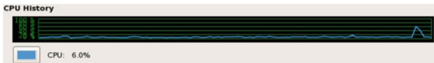
Fig. 23.5 Shows CPU usage after defending ICMP Smurf attack on the server
