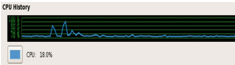
Fig. 23.4 Shows CPU usage on the server when the server was affected by ICMP Smurf attack
