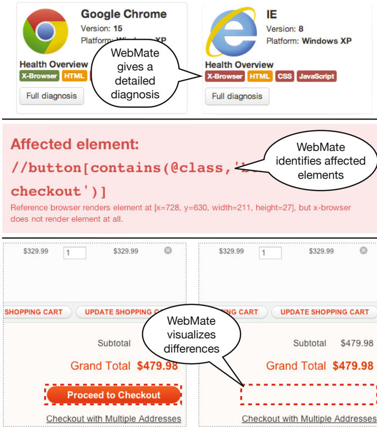
Fig. 3. Example of a diagnosis produced by WEBMATE. In Internet Explorer 8, the checkout button is missing. WEBMATE identifies the missing element and visualizes the problem using screen shots.
