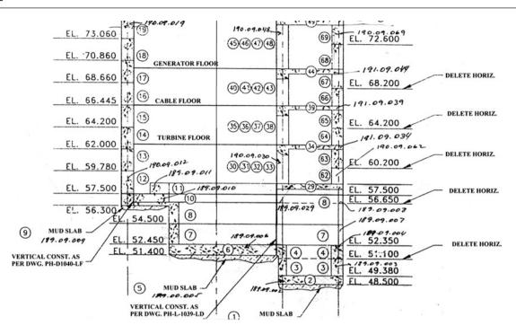
Fig. 17.1 As-built drawings for powerhouse structure
