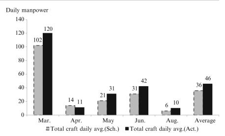
Table 16.11 Scheduled man-hours breakdown, distribution and daily average - Construction of a chemical plant
