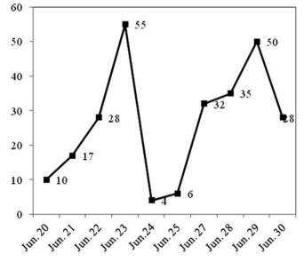
**Fig. 16.19** Graphic of rock blasted daily in the first 10 days of operation – Forecasting average daily a vance and prediction for a road project
