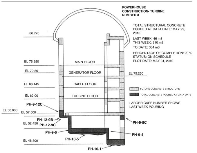
Fig. 16.11 Graphic information on work done for the foundation for a Pelton hydroelectric turbine – Observe also the tailrace, or discharge channel from the turbine
