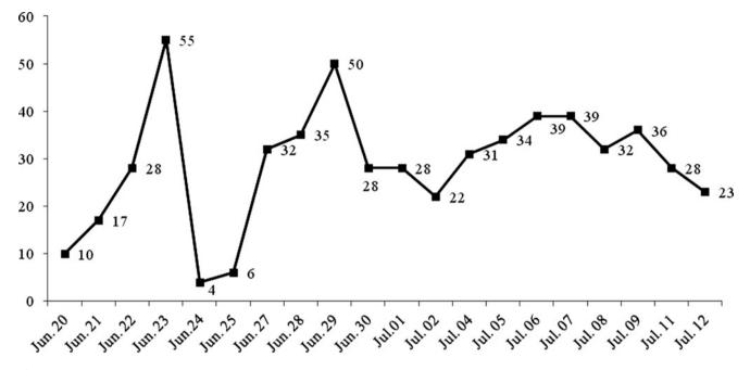
Fig. 16.20 Rock blasted daily in the first 20 days of operation - Forecasting average daily advance and prediction for a road project
