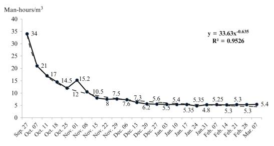
Fig. 16.13 Learning curve depicting relationship between man-hours and cubic metres of rock in boring a subway tunnel
