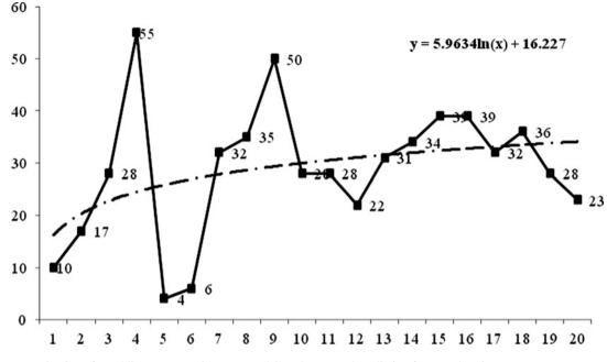
Fig. 16.23 Determination of trend line - Forecasting average daily advance and prediction for a road project
