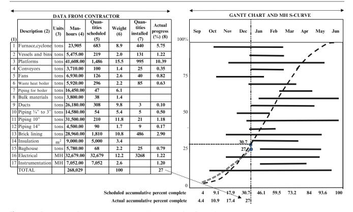
Fig. 16.14 Gantt chart and S-curve - Man-power control in the construction of a chemical plant
