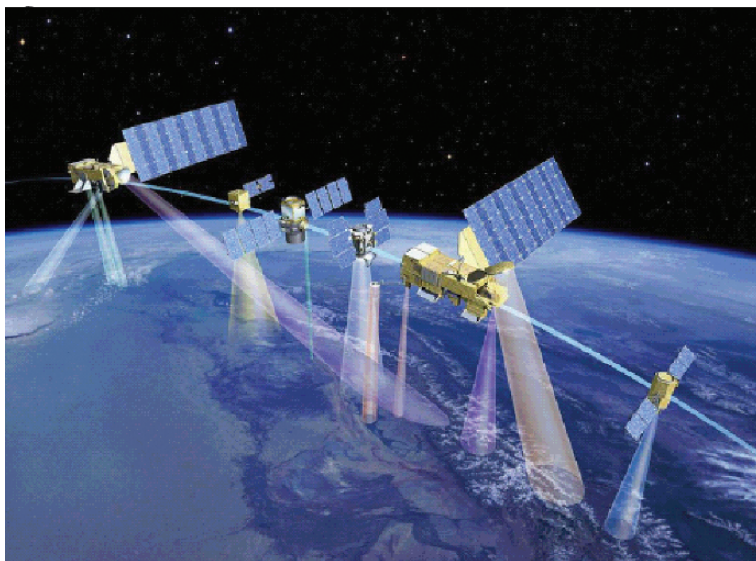
Fig. 5.8 The A train: a constellation of satellites that jointly measure aerosol, clouds and precipitation properties. Photo from NASA collection
