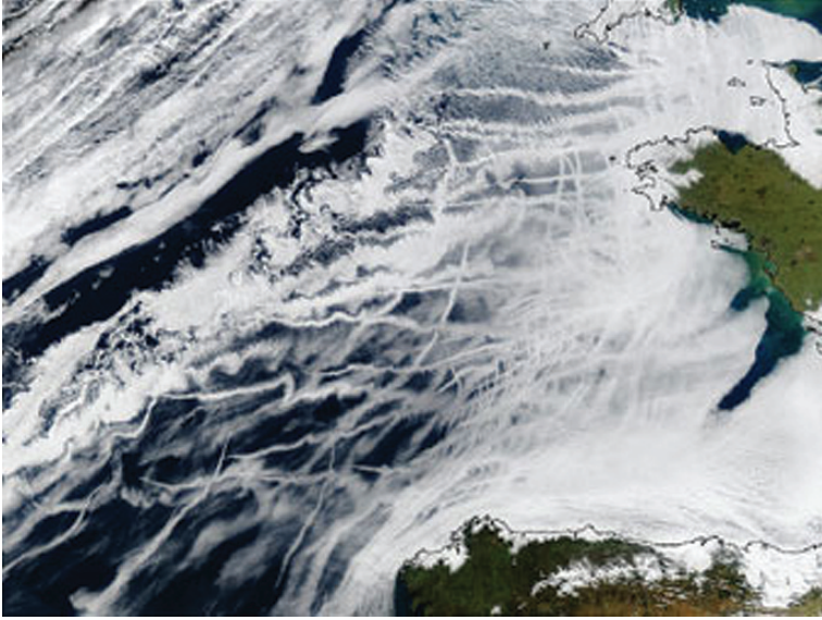
Fig. 6.11 Ship tracks off France. From bands 1, 4 and 3 of MODIS on the Aqua Satellite (Courtesy of NASA)
