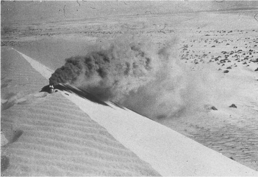
Fig. 6.29 Wind flow diversion of the lee slope of a seif dune demonstrated by smoke. Note the separation of flow at the crest, the reattachment on the lee slope and the diversion at the reattachment line
