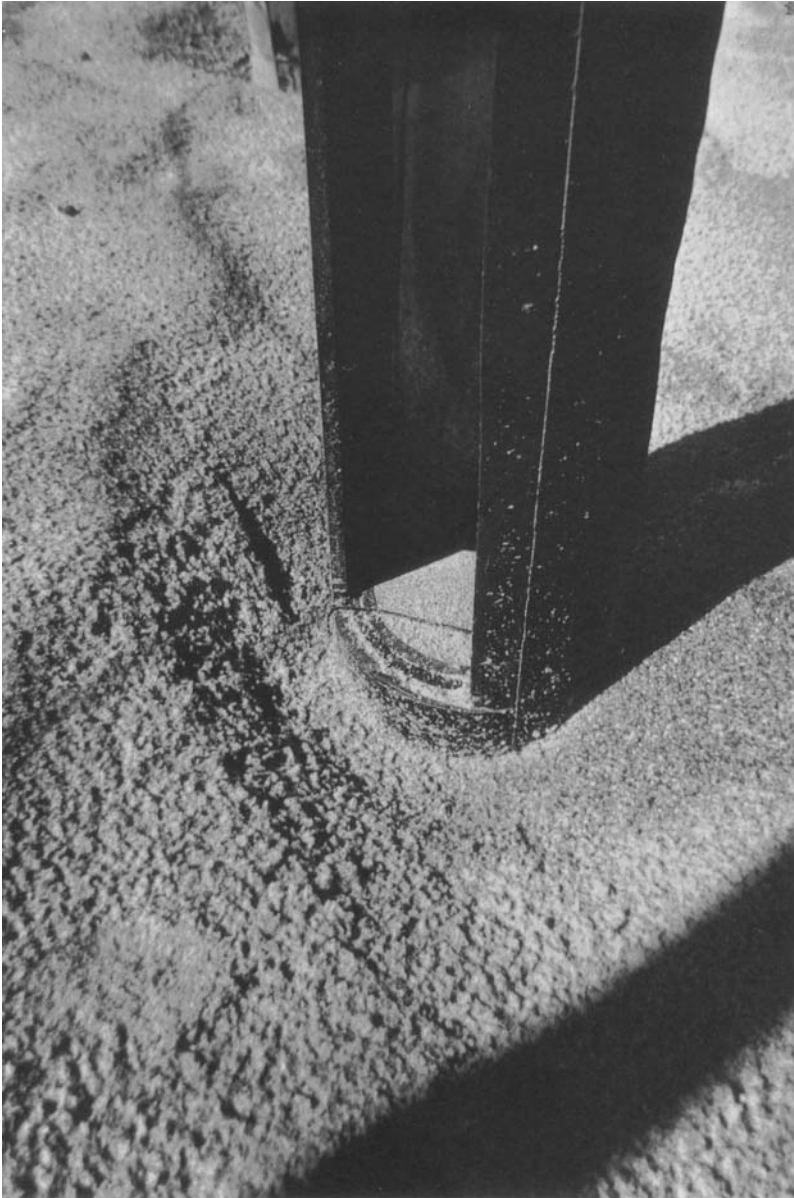
Fig. 10.8 Scouring around the base of a modified Leatherman trap. Note that the collector is full to the brim and that scouring has occurred from a wind direction not directly facing the trap's aperture. (Photograph by D. Blumberg)
