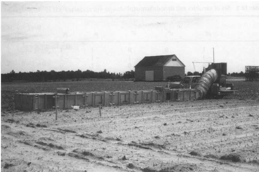
Fig. 10.2A,B Open-floored wind tunnel used in the field to determine the threshold shear velocities of natural sediments and soils. (Photograph by W. G. Nickling)
