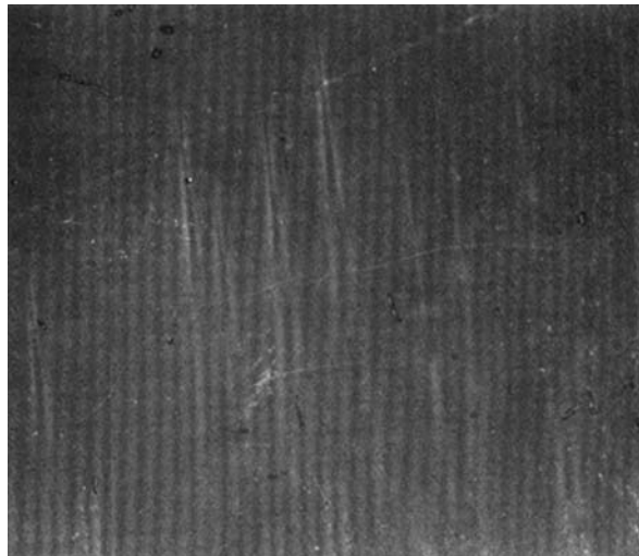
Fig. 2.2.6 180^\circ domains in \text{BaTiO}_3 crystal seen in polarized light during their growth. The polar axis is parallel to the wedges. The width of wedges at their base is about 6 \mu\text{m} . Reprinted with permission from Kobayashi (1967). Copyright (1967), Wiley-VCH Verlag GmbH & Co. KGaA
