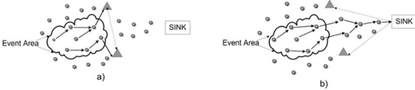
**Fig. 2** a) Automated and b) Semi-automated Architecture [5]
