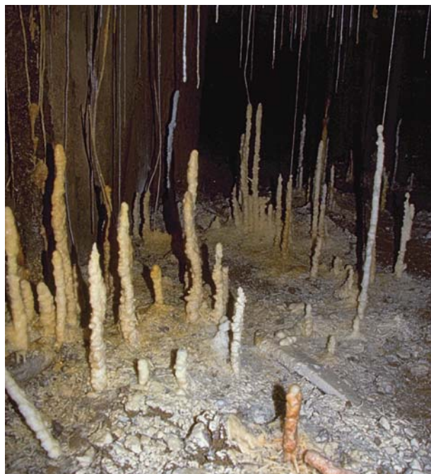
Fig. 7. Epsomite ( \text{Mg}[\text{SO}_4]\cdot 7\text{H}_2\text{O} ) stalactites and stalagmites in the Idrija/Slovenia mercury mine (the stalagmites are about 1 m high). Secondary minerals, such as epsomite, are dissolved during the flooding of the mine and – especially during the first flush – contribute to the acidity and metal content of the mine water.
