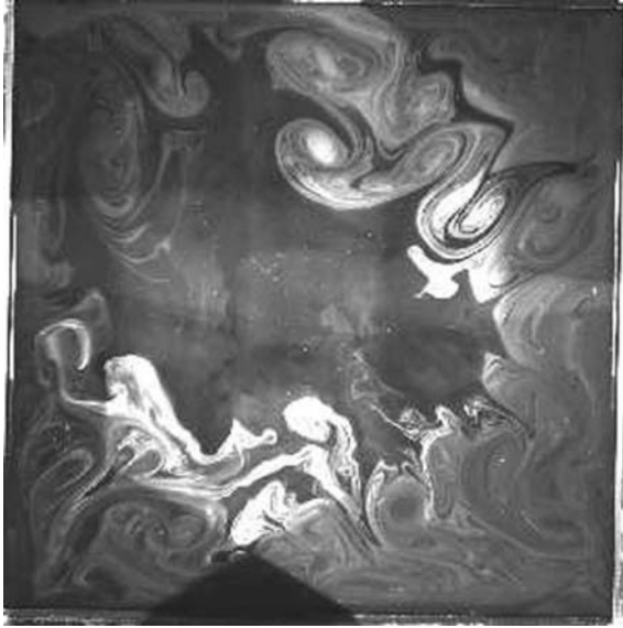
Fig. 4. A photograph taken approximately four oscillation periods after dye has been released for an experiment with \mathcal{F} = 2.09 ( Re = 15,000 ). In contrast to the previous figure the dye is not well mixed and has only been transported around the perimeter of the tank. This is due to the forcing parameters having \mathcal{F} > 1 so that dipoles could not efficiently form
