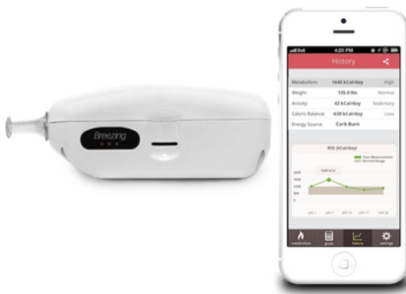
FIGURE 4.2 Breezing metabolic tracker that can wirelessly transmit data through Bluetooth to personal smartphone for resting metabolic rate monitoring. Reproduced with permission of Breezing Co.
