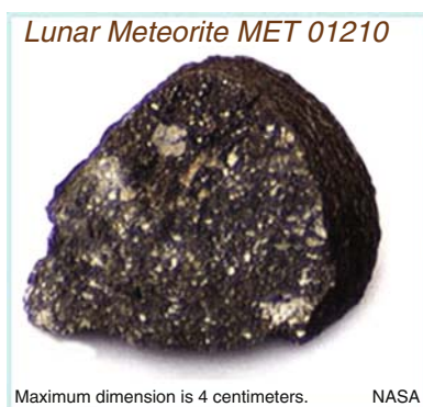
Fig. 15.3. Lunar meteorite MET 01210. A basaltic regolith breccia, it was collected in 2001 in the Meteorite Hills, Antarctica, and described in the Antarctic Meteorite Newsletter, 27, No. 1, Feb. 2004. It is composed mainly of very-low-titanium crust, which can be seen at the right. It is basically a collection of stone and mineral clasts or fragments in a glassy matrix. NASA photo, curator.jsc.nasa.gov/antmet/amn/amn.cfm . See color Plate 22
