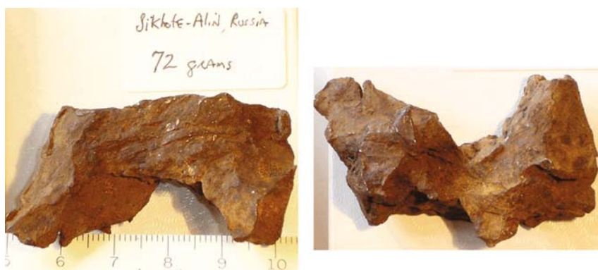
Fig. 15.5. A fragment of the Sikhote-Alin meteorite fall in eastern Siberia, February 12, 1947. It is classified a Type IIAB iron, coarsest octahedrite, with bandwidth of 9 mm. The circumstances of this spectacular meteoritic fall are described by Fessenkov (1955). See also color Plate 24
