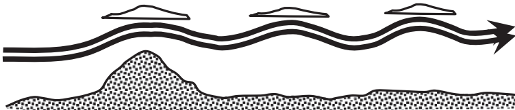
Fig. 10.29. Air flow over a mountain, illustrating oscillations at the Brunt-Väisälä frequency. Clouds often form when the air rises and cools, and evaporate when it sinks and heats, thus outlining the tops of the waves
