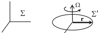
Fig. 10.2. A vector, \mathbf{r} , fixed in a rotating frame of reference, \Sigma' , and viewed from an inertial frame, \Sigma
