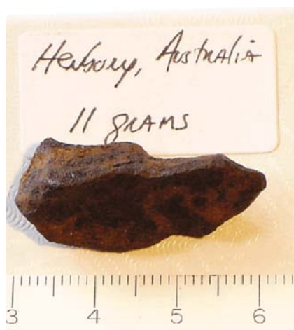
Fig. 15.4. A fragment of the Henbury iron meteorite find from the Northern Territory, Australia, 1931, according to the Bethany Sciences Company. It is classified as a medium octahedrite (IIIAB), with bandwidth 0.9 mm. See Plate 23
