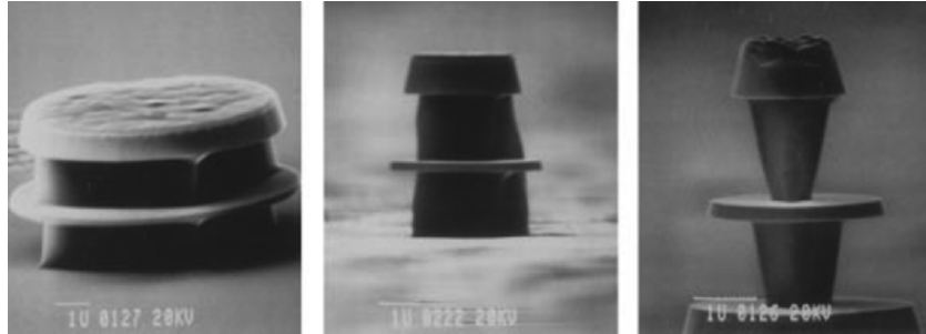
Fig. 6.7. WGM disk injection lasers with diameters of 8, 3, and 2 \mu\text{m} (from left to right ).
