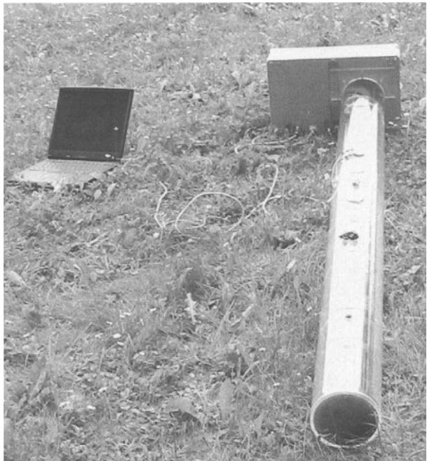
Figure 2 Plexiglas tube with the electronics box on top. The length of the tube is about 2 m, with a diameter of about 20 cm.
