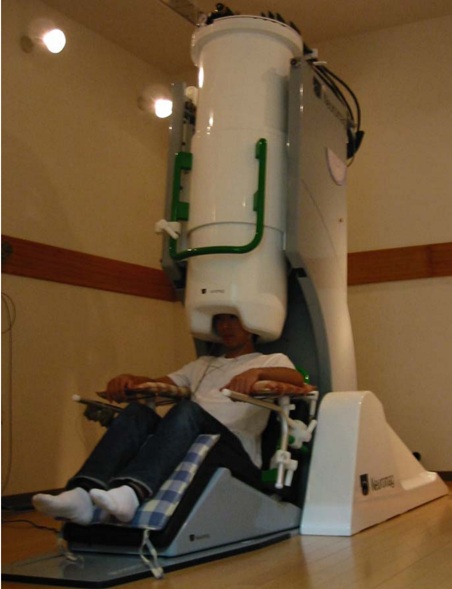
Photo 4.1 Magnetometer used in recording the MEG
