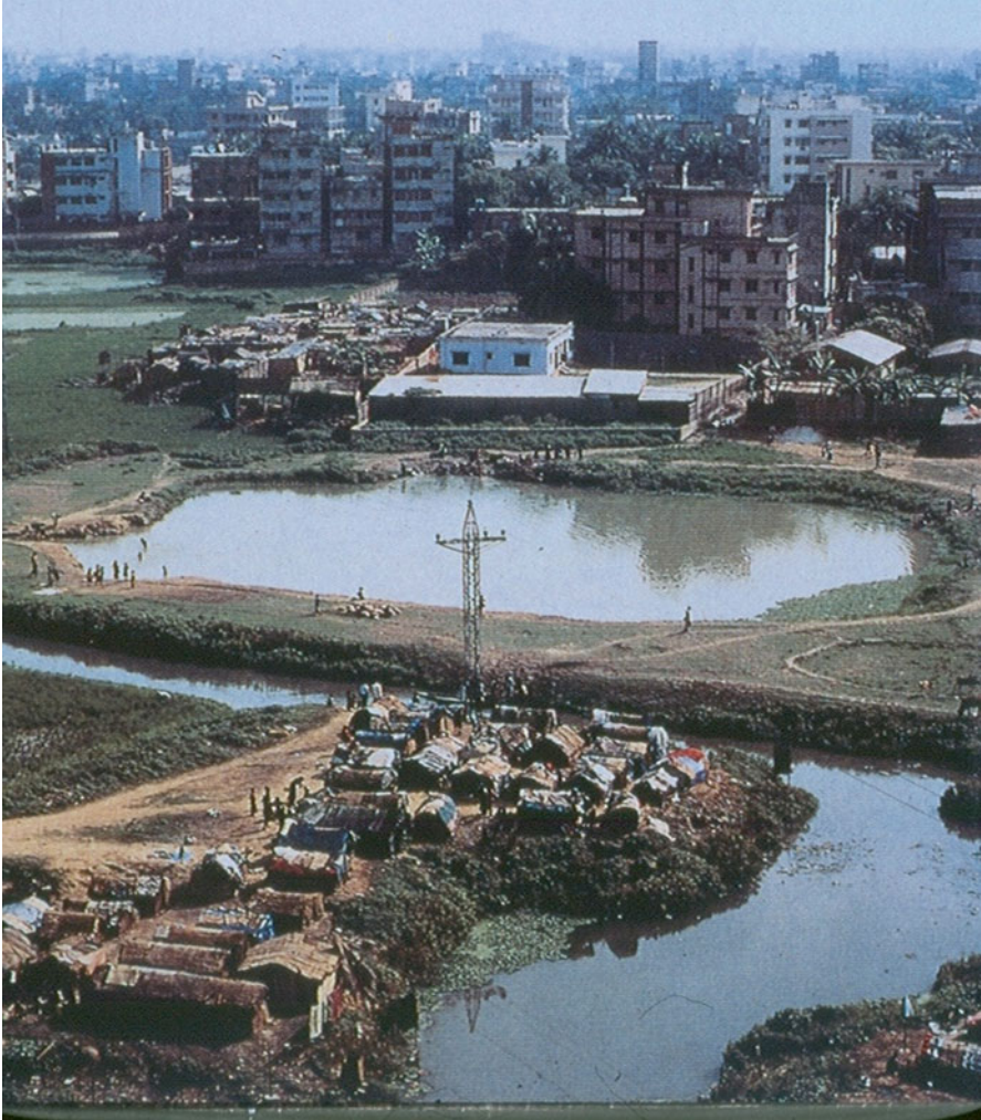
Fig. 6.7 Excavation of agricultural soils for brick production near Dhaka/Bangladesh (in the foreground, excavation ponds and brick production in mobile furnaces; in the background, houses constructed with bricks)
