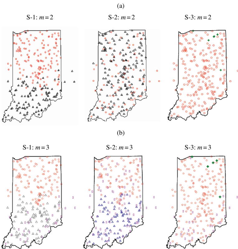
Fig. 4.3.3 Location of plausible hydrologic regions in Indiana obtained from 1-D SOFM. m denotes the number of output nodes of SOFM; S-1, S-2 and S-3 represent Scenario-1, Scenario-2 and Scenario-3 respectively. Each of the symbols in the diagram characterizes different clusters
