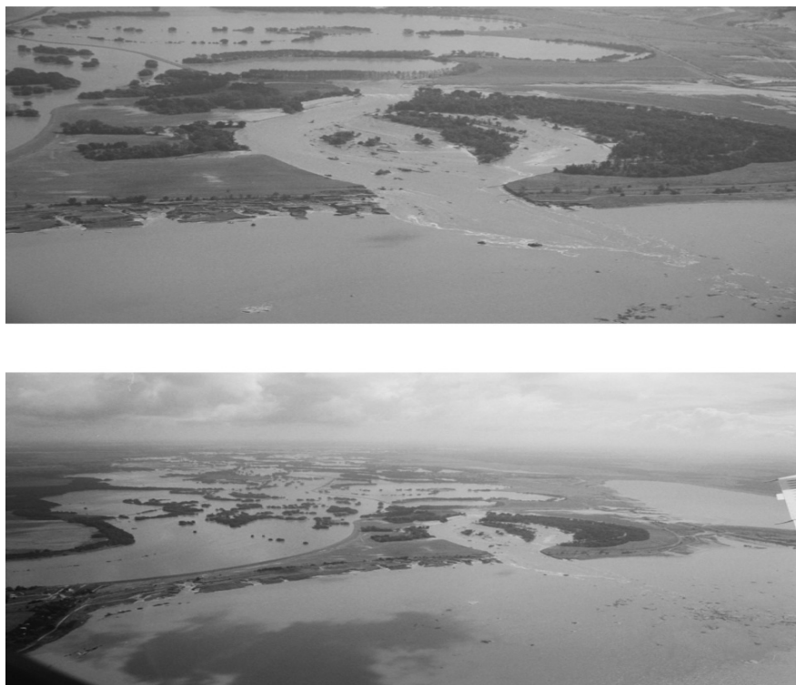
Fig. 1 a. Aerial picture of the breakthrough of the Mulde River at high water stand into a former open pit mine area at Goitsche on 15 August 2002; b. Similar to Fig. 1a but taken from a different aerial perspective to show the larger region covered by the floodwater breakthrough
