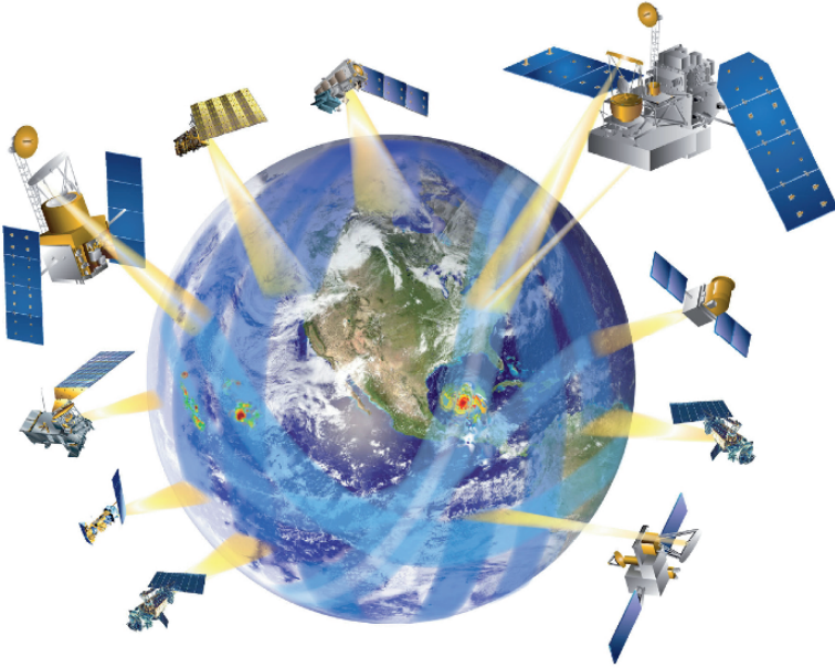
Fig. 3. The GPM Mission configuration with Core Spacecraft ( upper right ), the NASA Constellation Spacecraft ( middle left ) and partner constellation satellites providing global coverage
