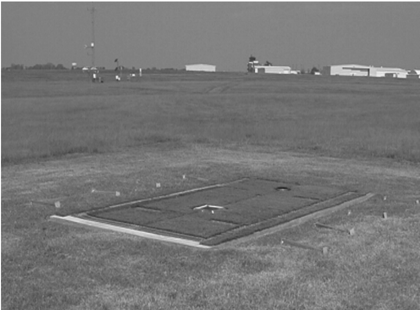
Fig. 3. View of pit with Geonor orifice at far end and 2dvd orifice at near end
