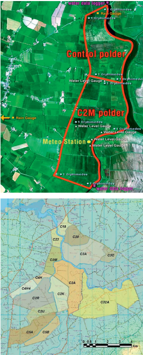
Fig. 33.2 The pumped [C2M] and control [C23] polders in the top left corner of the set of 15
