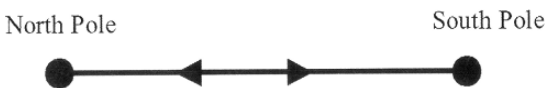
Fig. 5.9. Force of attraction between a north and a south pole placed at a distance r
