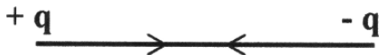
Fig. 4.1. Coulomb force of attraction between a positive and a negative charge separated by a distance r
