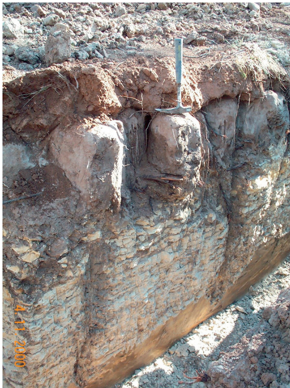
Fig. 2 The study soil with characteristic columnar peds in the B horizon. Note the fractures penetrating into the thinly bedded lithic sandstone (Jurassic, Pilliga Sandstone)
