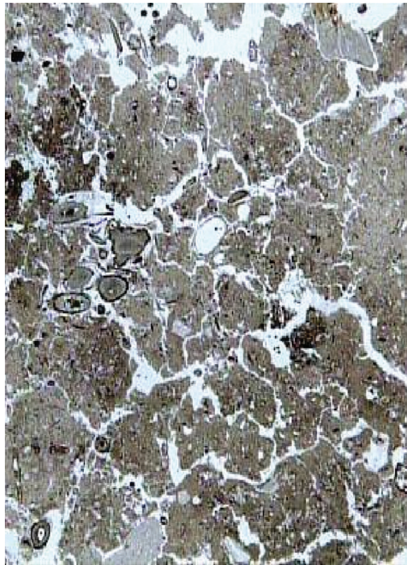
Fig. 4 Microphotograph of a vertically oriented soil thin section prepared from undisturbed samples from the surface layer (0–100 mm) of a loam soil (Lamelli-Calcaric Cambisol, according to FAO-IUSS-ISRIC classification, 1998) cropped with maize, showing an example of subangular blocky structure, where the aggregates are separated and surrounded by elongated continuous pores. The white areas represent the pores. Frame length 3 \times 5 mm
