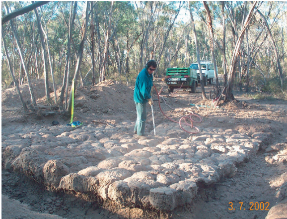
Fig. 4 Columnar peds exposed after removing the topsoil by air-blasting. The mallee, (multi-stem habit) of Eucalyptus viridis , is clearly evident. Southeast quadrant
