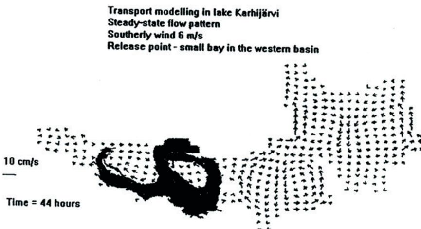
Fig. 6: Particle paths as calculated by the 2DH-J Karhijärvi model.
