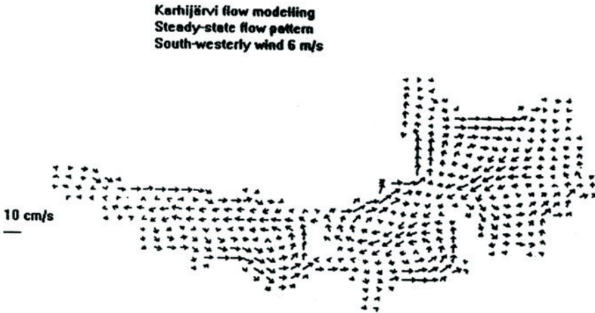
Fig. 4: Calculated circulation pattern in Karhijärvi.
