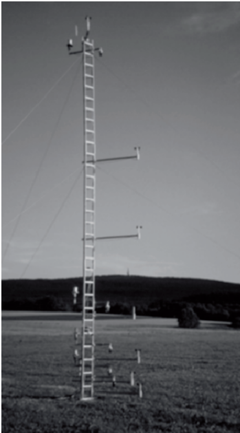
Fig. 4.8. Measuring mast for profile measurements (Photograph: Foken)
