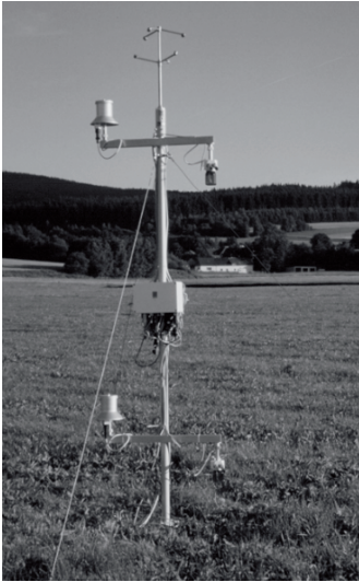
Fig. 4.7. Measuring system for the modified Bowen-ratio method (METEK GmbH Elmshorn and Th. Friedrichs & Co. Schenefeld near Hamburg; Photograph: Foken)
