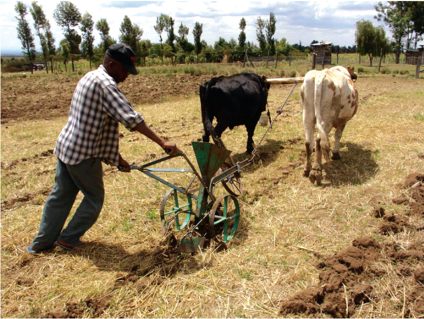
Fig. 4.8 Small-scale version of conservation agriculture in Kenya. Direct seeding of maize (after wheat) and fertilizer application is done in one pass by a locally manufactured implement. Weeding needs an extra application with herbicides or manual weeding
