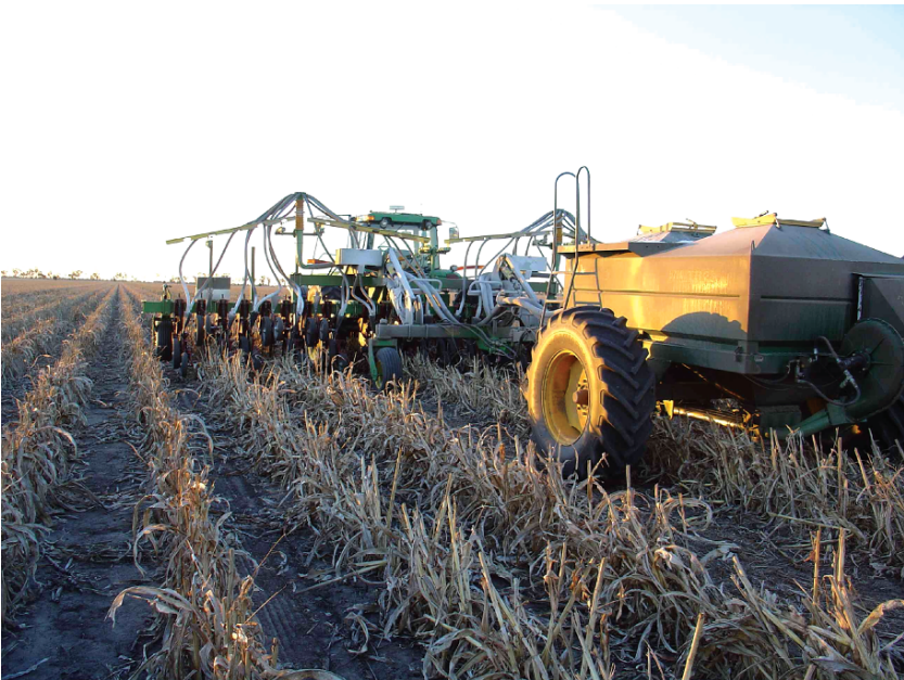
Fig. 4.9 Computer- and satellite-driven direct seeder for precision conservation agriculture in Australia, including herbicide application only where green weeds are detected by a sensor, where seeding is done and fertilizers applied according to the satellite information about soil fertility and previous yields
