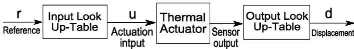
Fig. 10.15 Block diagram of the open-loop control system including input and output look up tables, reference, electrothermal actuator and sensor [39]
