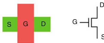
Poly crossed over Diffusion → Field effect transistor (FET)
