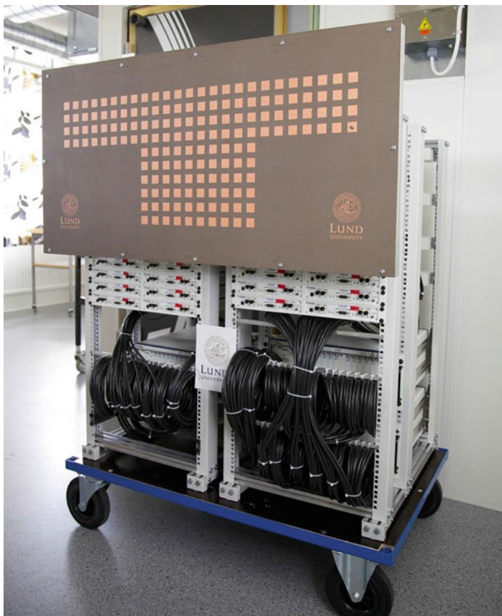
Fig. 7.2 LuMaMi: Lund Massive MIMO Test-bed [17]
