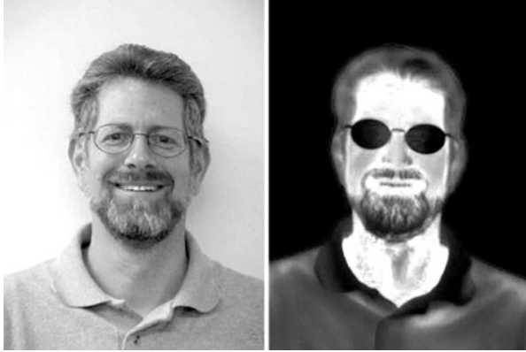
Fig. 4.47 Photographs in visible light and IR thermal radiation that is naturally emanated from the object. Note the brighter (appearing warmer) areas at wrinkles and skin folds near nose—a result of cavity effect. Eyeglasses appear black (cold) because glass is opaque in mid- and far-infrared spectral ranges and does not pass thermal radiation from eyes. (Photo: courtesy of Infrared Training Center , www.infraredtraining.com )
