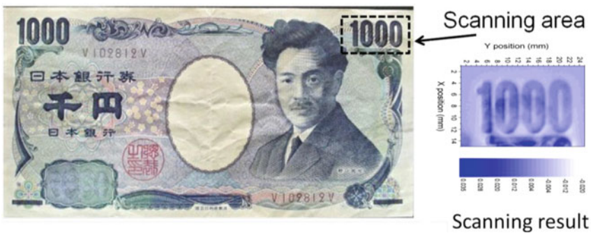
Fig. 8.13 Scanning result of Japanese 1000 yen bill using the GMI field sensor (reprinted with the permission of MDPI [33])
