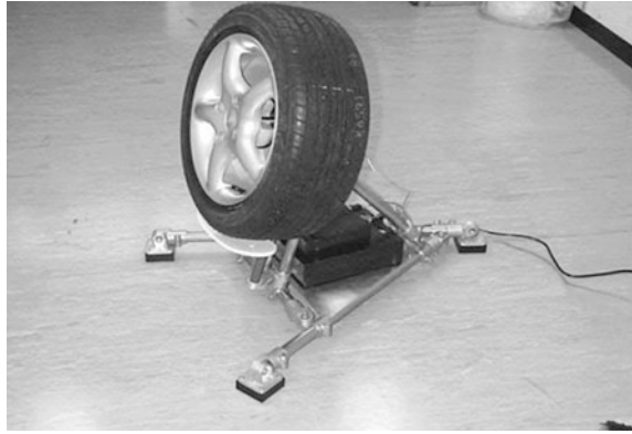
Fig. 8.17 Tyre pressure monitoring system incorporating an amorphous alloy wireless, battery-free sensor (reprinted with the permission of Elsevier [17])
