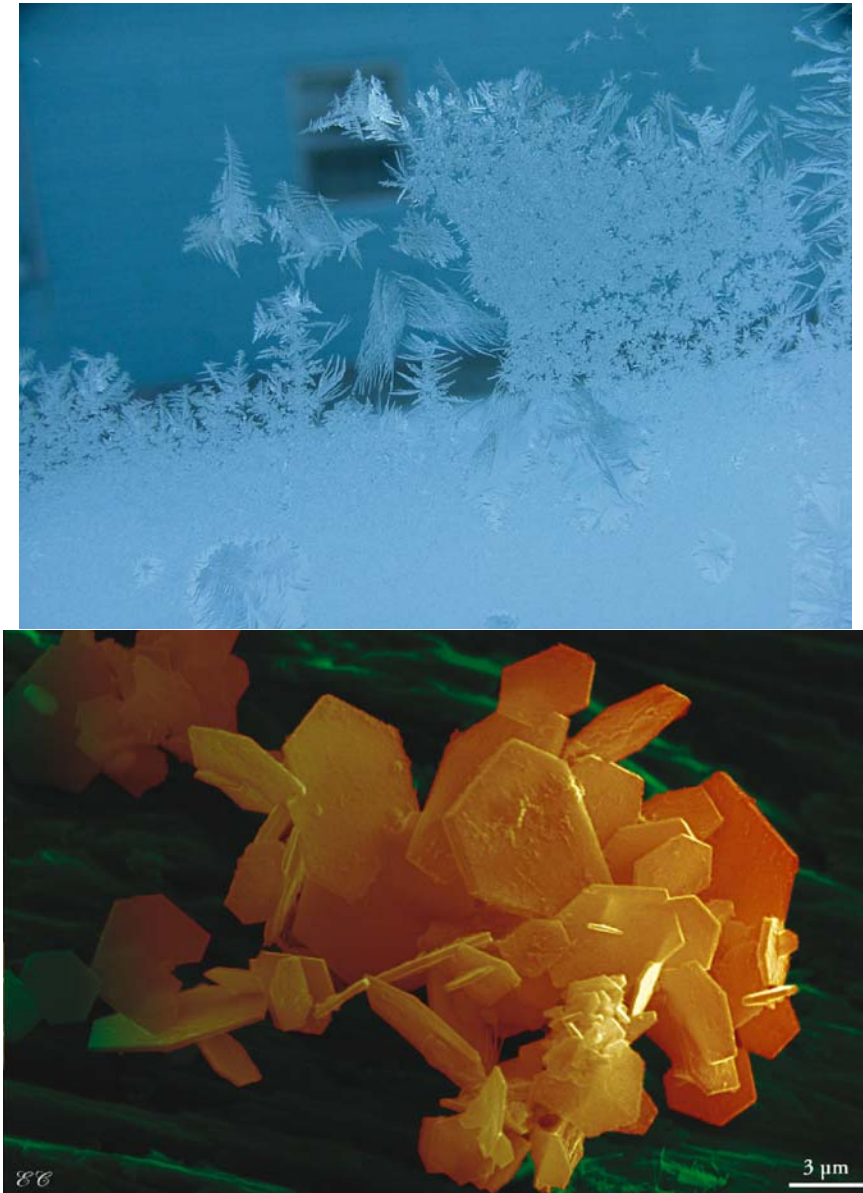
Fig. 7.1 Crystals formed in natural and laboratory settings; (a) ice crystals grown on a glass window (Benning unpublished image) and (b) hexagonal pyrrhotite platelets grown from an iron sulphide precursor at 200°C; the growth followed a solid state process (see also Hunger and Benning, 2007; image Benning, unpublished, the copyright for the colour image (b) in the online version of this chapter is copyrighted to Eric Condliffe, Leeds)
