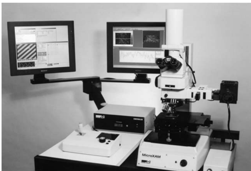
Fig. 3.12 Current generation vertical scanning interferometer. MicroXAM instrument, similar to that used to produce the VSI data within this paper (ADE-Phase Shift). This instrument utilizes Mirau optics, and was originally developed for purposes of quality control metrology in the semiconductor industry. Scanning interferometers permit high resolution, non-contact, rapid scanning-mode data acquisition of crystal surfaces, together with sophisticated data reduction and filtering routines ( http://www.phase-shift.com/products/microxam.shtml )
