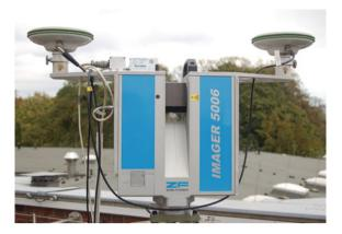
Fig. 1 Prototypical realization of the MSS formed by a laser scanner (blue) and two eccentrically mounted GNSS antennas (green). This MSS was used for the field experiment
