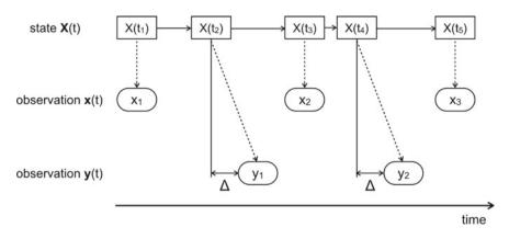
Fig. 4 A diagram that describes the data generation process. The observed data  $x_i$  and  $y_j$  are generated from a latent light curve  $X(t^{\Delta})$  representing the unknown true magnitudes evaluated at discrete observation times
