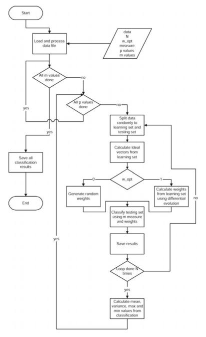
Fig. 2 Simplified flowchart of the classification procedure
