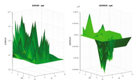
Fig. 5 Error measure in the identification of AP6, for 74,505 values of the pair  $(na, \lambda)$ . Plot on the right shows the same plot on the left after applying a correcting function that highlights the maximum and minimum peaks, maintaining the proportion among all the points, in order to show a better display
