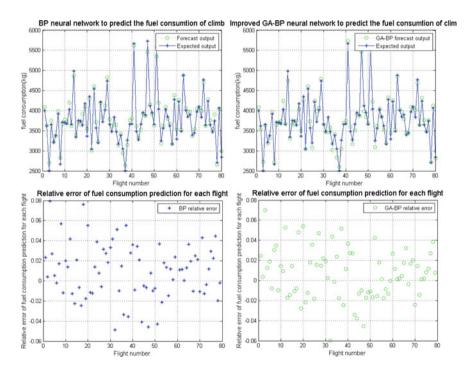
Fig. 2 Output and relative error of model prediction
