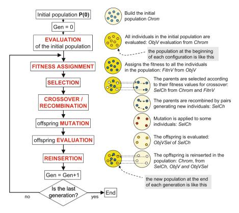
Fig. 6 Scheme of the genetic algorithm used in this work
