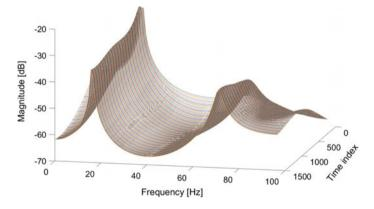
Fig. 4 Power spectral density of the time-variable AR(6) model
