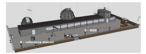
**Fig. 2** Location of the practical experiment on the roof of the building of the Geodetic Institute (Messdach) at the Leibniz Universität Hannover, Germany. The MSS from Fig. 1 is mounted on pillar 5 while reference station is located at pillar 8
