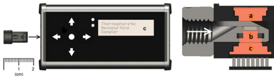
Fig. 12 The thermal precipitation sampler (TPS): the overall device including the removable sample cartridge ( left ). Right : view of the TPS region containing the hot plate (a), TEM grid holder (b), and cold plate (c) [61]
