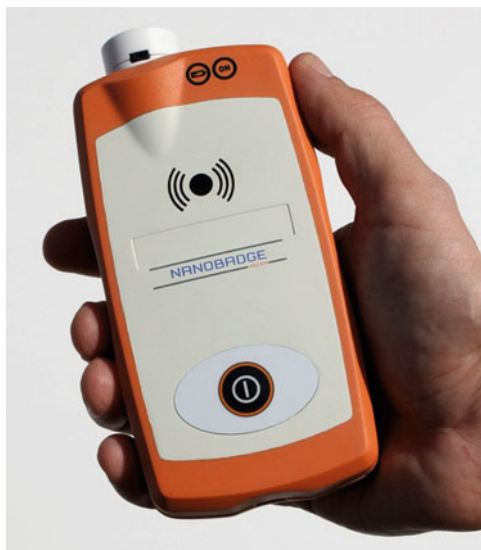
Fig. 13 The NanoBadge; the white cassette on the top of the device is equipped with a sealed track-etched membrane to collect airborne particles; a single on-off switch makes the device robust and very simple to use
