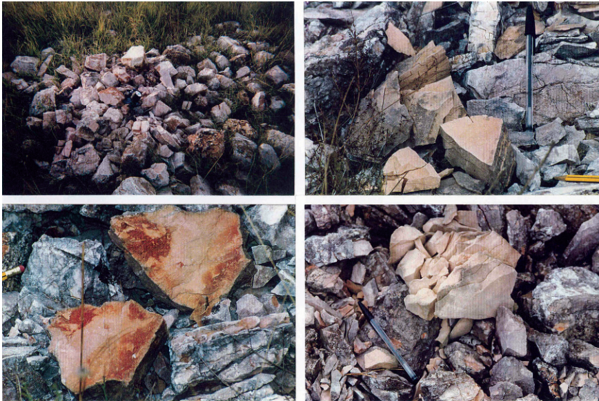
Fig. 6 General typical view of a rock pile ( upper left ) and three detail views near the heavily-damaged village of Annifo following the Colfiorito earthquake. Most of the stones in the piles (fragile marly limestone) were freshly fractured or broken (After Bouchon et al. 2000)
