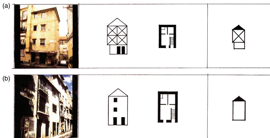
Fig. 13 Constructive typologies used before the earthquake: a) house of narrow front with an external wall forming a “bump”; b) house of narrow front with a roof of “four attics”
