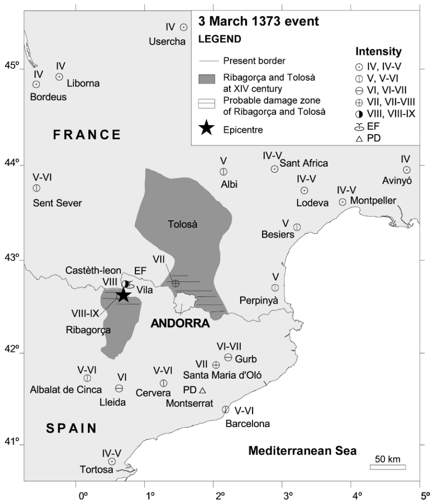
Fig. 2 Intensity map (EMS-98) for the earthquake of 3 March 1373 and macroseismic epicentre. PD = probable damage and EF = effects on springs
