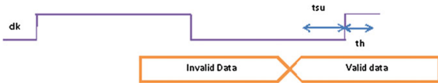
Fig. 11.2 Valid setup time region timing sequence
