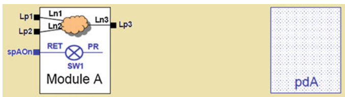
Fig. 14.15 Power switch creation [2]
