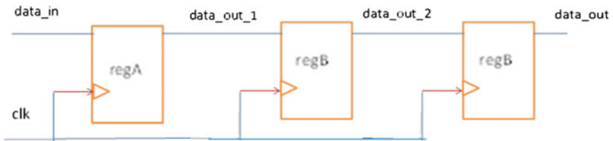
Fig. 13.9 Synthesis result for the three-stage level synchronizer
