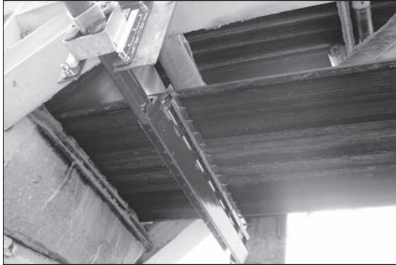
Figure 17. Scrapers replaced many times
