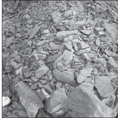
Figure 17. Typical tunnel muck showing crushed blocks from open mode operation
