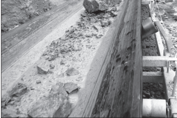
Figure 21. Water and boulders on the conveyor
