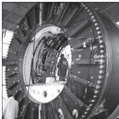
Figure 11. Original size shop test of the main drive seal system
