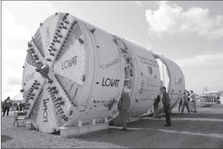
Figure 3. Mercer Street tunnel EPB TBM
