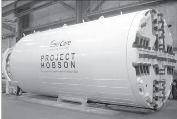
Figure 2. Earth pressure balance TBM during factory testing
