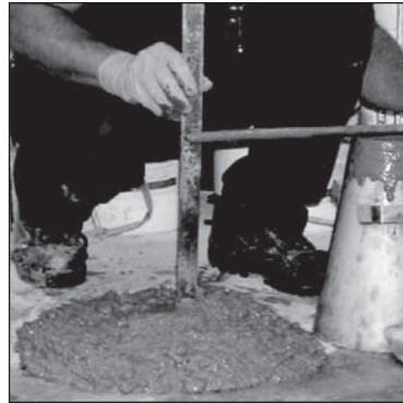
10% HDLS added by wt, 8.5" slump
