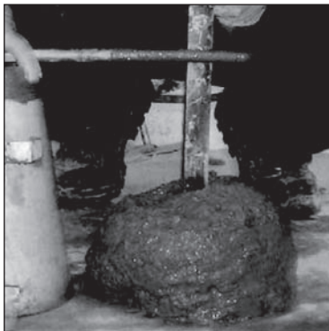
FIR 30%+50ml P2+HDLS, 6.5" slump
