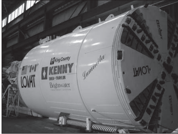
Figure 2. Brightwater East Lovat TBM
