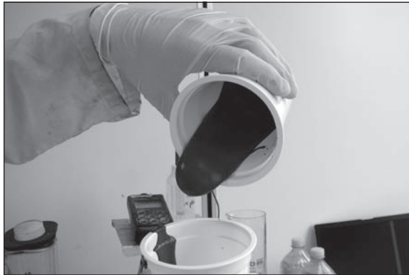
Figure 7. Component A gelled in the glass during the mixing
