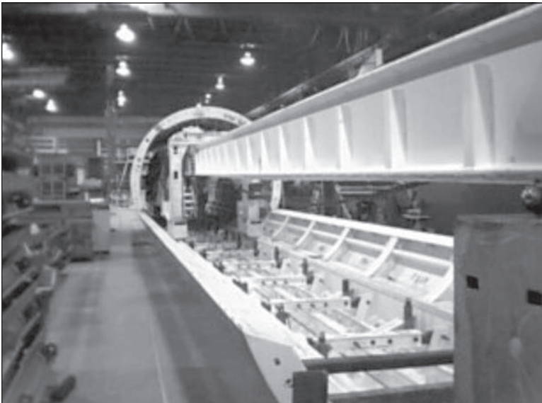
Figure 13. Shop testing of 3.05 meter (10 foot) diameter formwork with carrier
