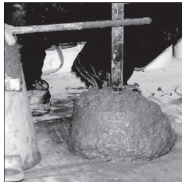
FIR 30%+65ml P2+LS slurry, 6.5" slump
