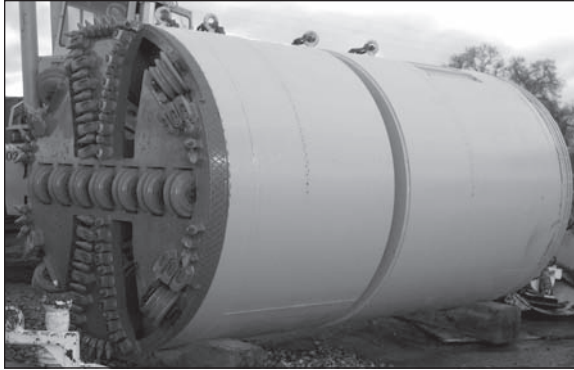
Figure 12. The MTBM used for the Mokelumne River crossing
