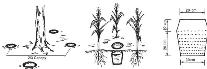
Fig. 5.9 Seepage irrigation for fruit trees and corn. a Four vessels around a tree, b One vessel for three plants, c Percolated porcelain vessel. Source Zhu et al. (2012)
