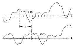
Figure 26: Time-shift of signals
