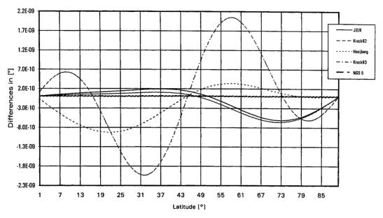
Figure 70: Round-trip error of the meridional arc in degrees
