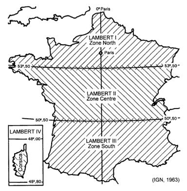
Figure 81: Lambert's conformal conical projection of France
