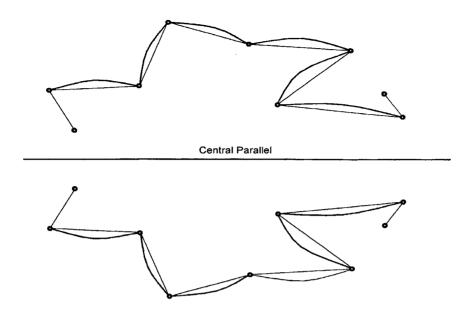
Figure 76: Normal Mercator and Lambert projection - projected geodetic vs. grid angles
