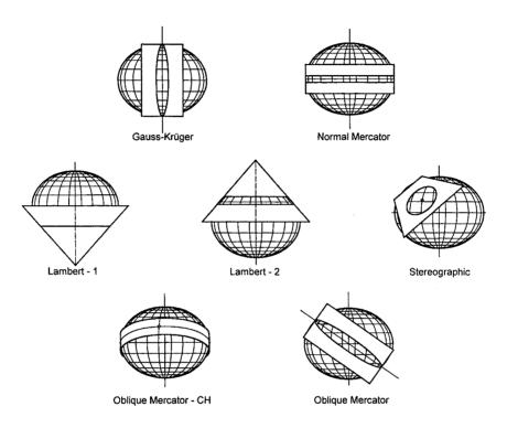
Figure 73: Tangency or secancy of various map projection surfaces
