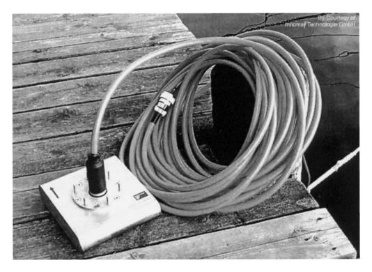
Figure 134: Innomar SES 2000 Compact - parametric transducer with cable
