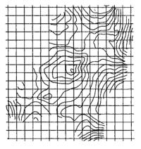
Figure 50: ED50 corrections for  $\Delta N$
