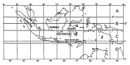
Figure 89: UM and UTM grid zones for the equatorial territory of Indonesia
