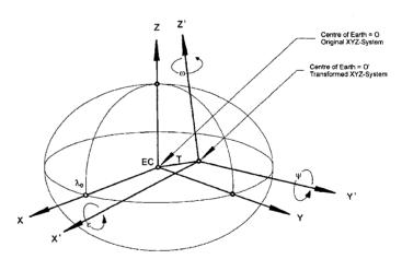
(earth-centred, earth-fixed) coordinates Figure 53: Translated and rotated 3D-coordinate system
