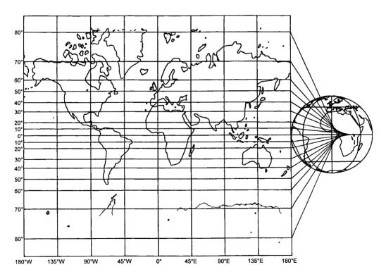
Figure 85: Mercator projection of the sphere
