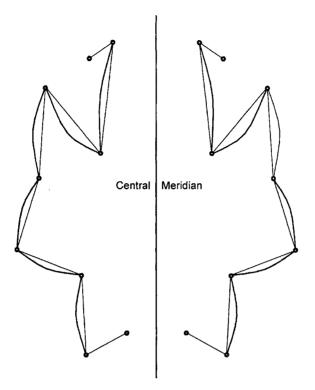
Figure 77: Transverse Mercator vs. grid angles
