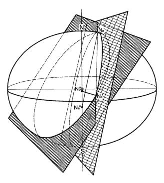
Figure 63: Normal sections and the reference ellipsoid
