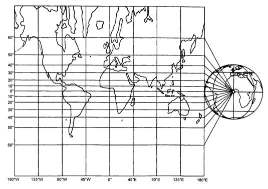
Figure 84: Perspective projection of the sphere
