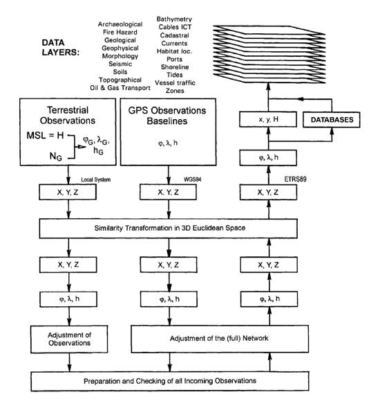
Figure 118: Sketch of spatial dataflow using multi-dimensional Databases and data Overlays in brief
