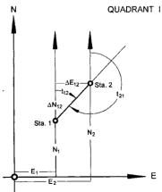
Figure 34: Bearing and distance
