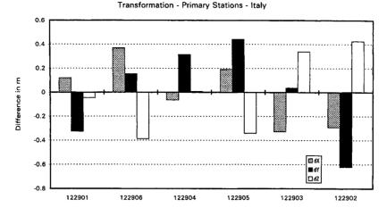
Figure 56: Calculated differences for the 6-parameter transformation solution
