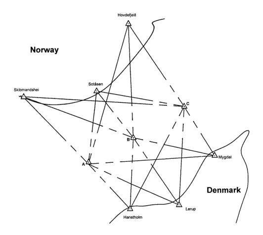
Figure 19: Flare triangulation of the connection Denmark and Norway
