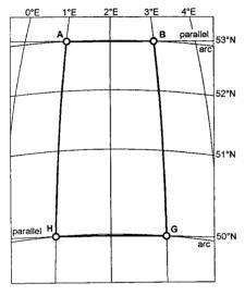
Figure 43: Ellipsoidal quadrilateral area
