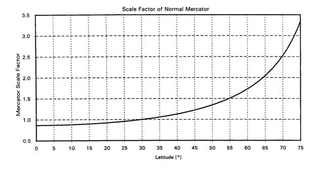
Figure 87: Scale factor as a function of 75° latitudinal zone width
