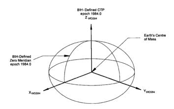
Figure 9: World Geodetic System of 1984 definition
