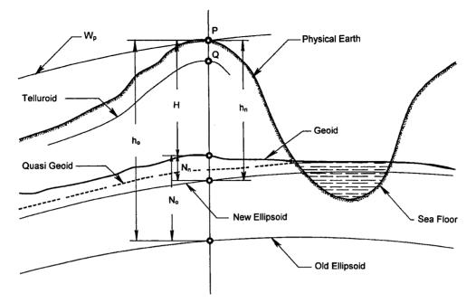
Figure 54: Geoid separation of the old and the new Datum
