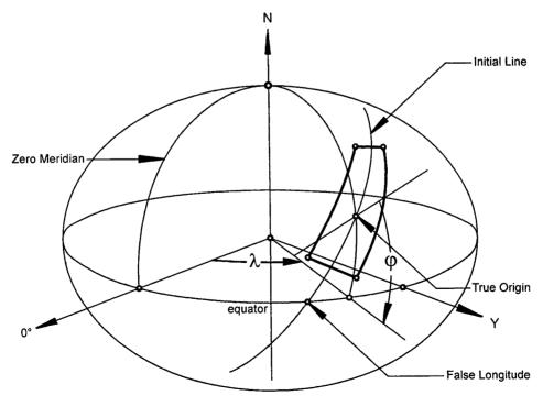
Figure 92: Initial Line of the Borneo RSO grid
