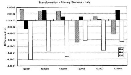
Figure 58: Calculated differences for the 9-parameter transformation solution
