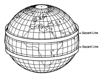
Figure 88: Normal Mercator with two secant lines
