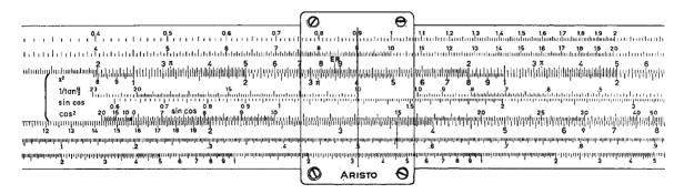
Figure 113: Part of the "Aristo-Geodät" slide rule in Gon
