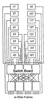
Figure 115: SP-Switch Circuitry
