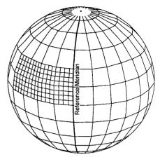
Figure 97: Polyeder mapping system
