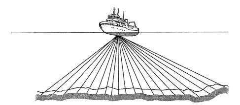
Figure 130: Hull mounted multibeam echosounder geometry
