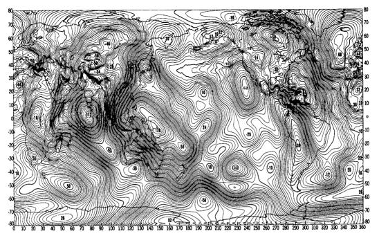
Figure 4: NASA/GSFC GEM4 - Global Detailed Gravimetric Geoid in the Miller projection
