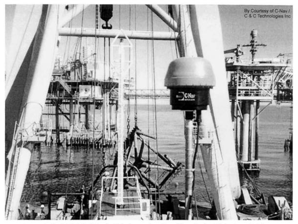
Figure 29: C-Nav Starfire GcDGPS World Receiver in the foreground on a barge lifting a Hurricane Katrina damaged platform
