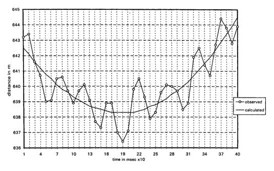
Figure 38: Determination of the shortest LS sum distance of Baseline A1
