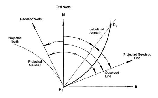
Figure 75: Azimuth and convergence
