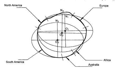
Figure 6: The geoid and three reference ellipsoids
