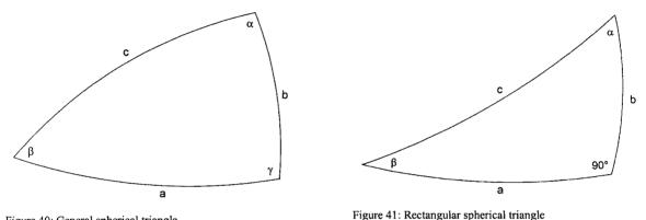
Figure 40: General spherical triangle
