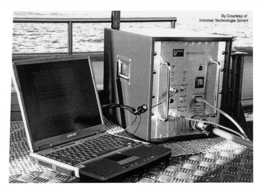
Figure 133: Laptop PC with Innomar SES 2000 Compact - parametric sub-bottom profiler
