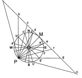
For a small country whose boundaries are contained in a small circle of a radius between three and six degrees, the stereographic projection is effective using the conformal Gaussian sphere. The scale is about unity at a distance of 170 kilometres from the central point.
