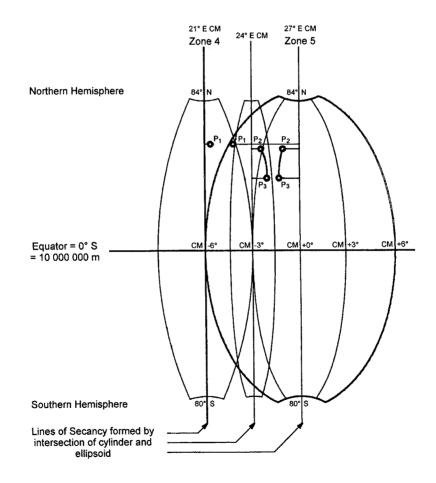
Figure 102: Conversion between 3° - 6° zone systems and 6° - 6° zone systems
