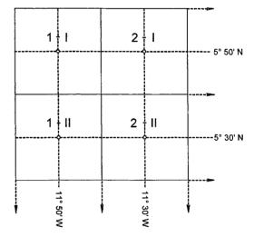
Figure 101: Part of the Indonesian Polyeder mapping system
