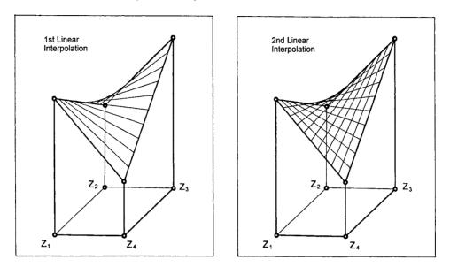
Figure 52: Cross sections of the bi-linear interpolation surface are defined by straight-line elements
