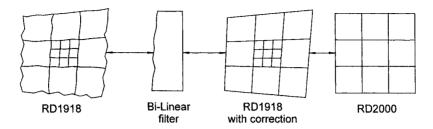
Figure 30: Distorted - filtered - transformed - corrected grids
