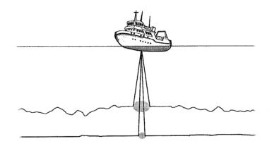
Figure 129: Hull mounted multibeam echosounder geometry
