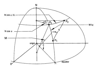
Figure 64: Geodetic triangle
