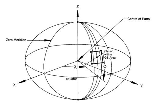
Figure 82: Gaussian sphere / ellipsoid mapping system
