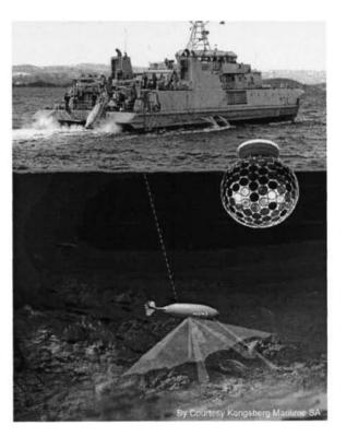
Figure 125: Hugin-3000 AUV using GNSS and Doppler log
