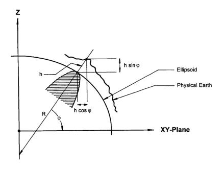
Figure 55: Ellipsoidal and physical Earth
