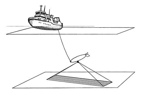
Figure 131: Towed Fish mounted sidescan sonar
