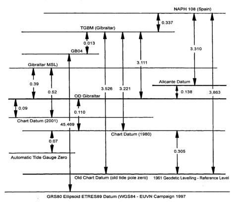
Figure 21: One example of various reference levels and vertical datums in use - Spain / Gibraltar
