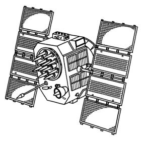
Figure 27: One of the first GPS-satellites
