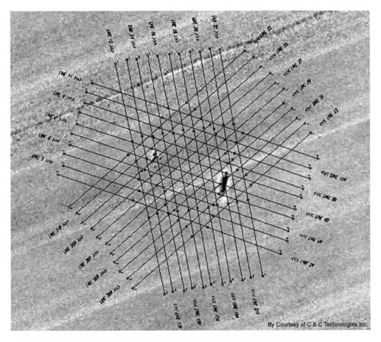
Figure 136: C&C side-scan sonar survey pattern for the German U-166 submarine in the Gulf of Mexico
