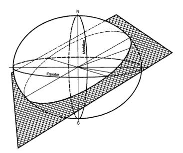
Figure 62: The great elliptic arc and the reference ellipsoid
