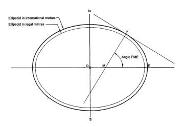
Figure 46: Bessel ellipsoids in legal metres and international metres
