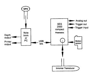
Figure 132: Sketch of DGPS surveying by parametric echosounder
