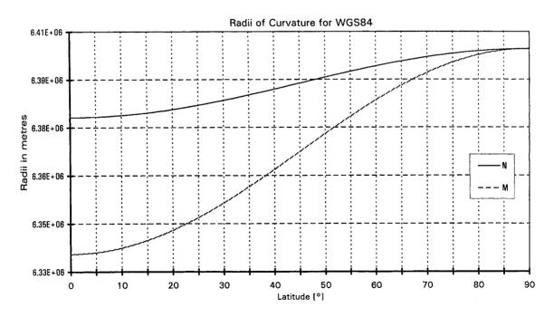
Figure 48: Radii of curvature in Prime Vertical and in the Reference Meridian
