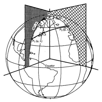
Figure 66: The geodesic and the reference ellipsoid
