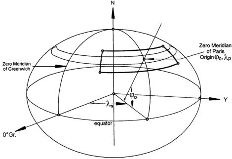
Figure 80: Lambert's conical IGN zone
