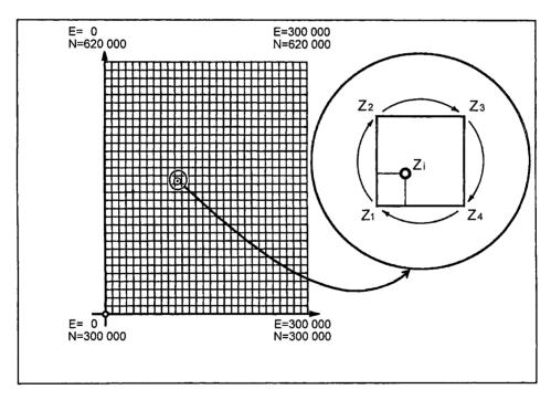
Figure 51: Location of a grid square for interpolation
