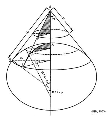
Figure 78: Lambert's conformal conical projection
