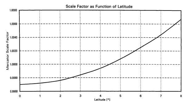
Figure 86: Scale factor as a function of 8° latitudinal zone width
