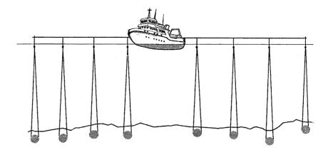
Figure 128: Simultaneous deployment of multi single-beam echosounders
