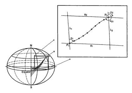
Figure 65: Geodesic divided into dS line elements
