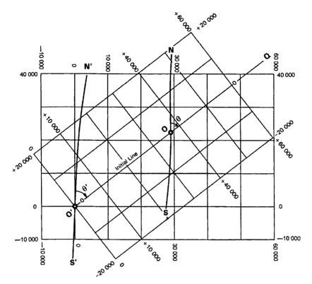
Figure 91: Borneo Rectified Skew Orthomorphic grid
