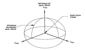
Figure 8: Parametry Zemli System of 1990 definition
