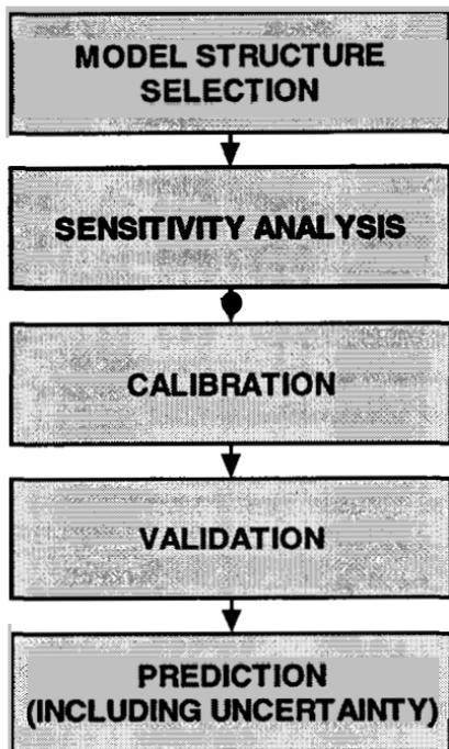
**Fig. 2.2** Conventional (simplified) procedure for local rainfall-runoff modelling
