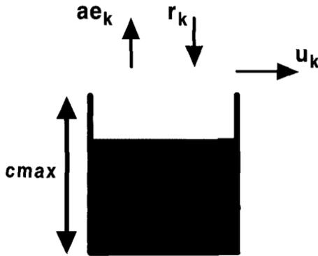
**Fig. 3.4** Single storage element defined by the size parameter  $c_{max}$ . The fluxes are actual evapotranspiration  $ae_k$ , rainfall  $r_k$  and effective rainfall  $u_k$ . All at time step  $k$ .
