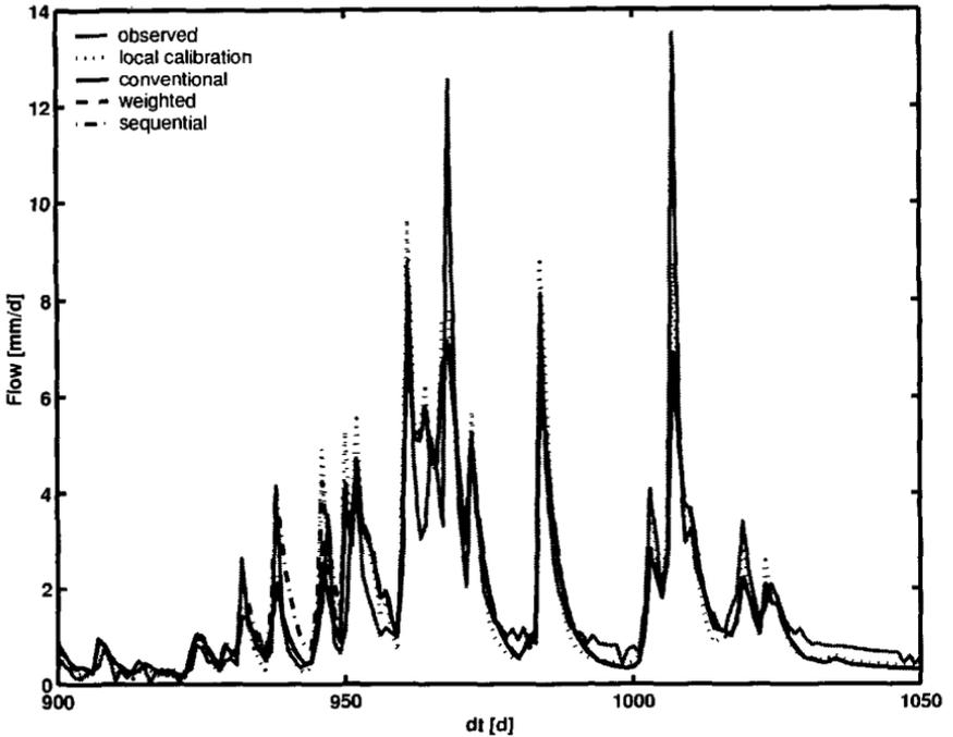
**Fig. 5.15** Flow prediction for the Teise @ Stonebridge using the different regionalized parameter values and the local parameter set that is optimum with respect to the RMSE. The top plot shows a high flow period on original scale, while the bottom plot is a low flow period on log-transformed scale.
