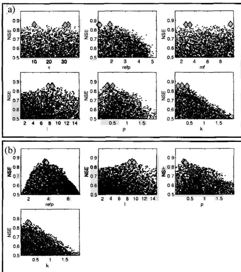
**Fig. A.3** Dotty plots comparing parameter identifiability of an initial complex model (a) and a final, simplified model (b) retaining only identifiable parameters, from the regionalization example. Note that the performances of simple and complex models are similar.
