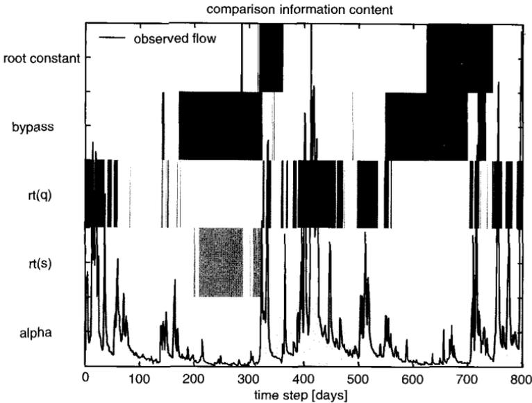
**Fig. 4.21** Comparison of the information content of a two-year period for the different parameter values (days 950 to 1750). Only time steps with an information content above 0.3, with respect to individual parameters, are shown in the different grey shades. (From Wagener *et al.*, 2003a; reproduced with permission of John Wiley & Sons, Inc.)
