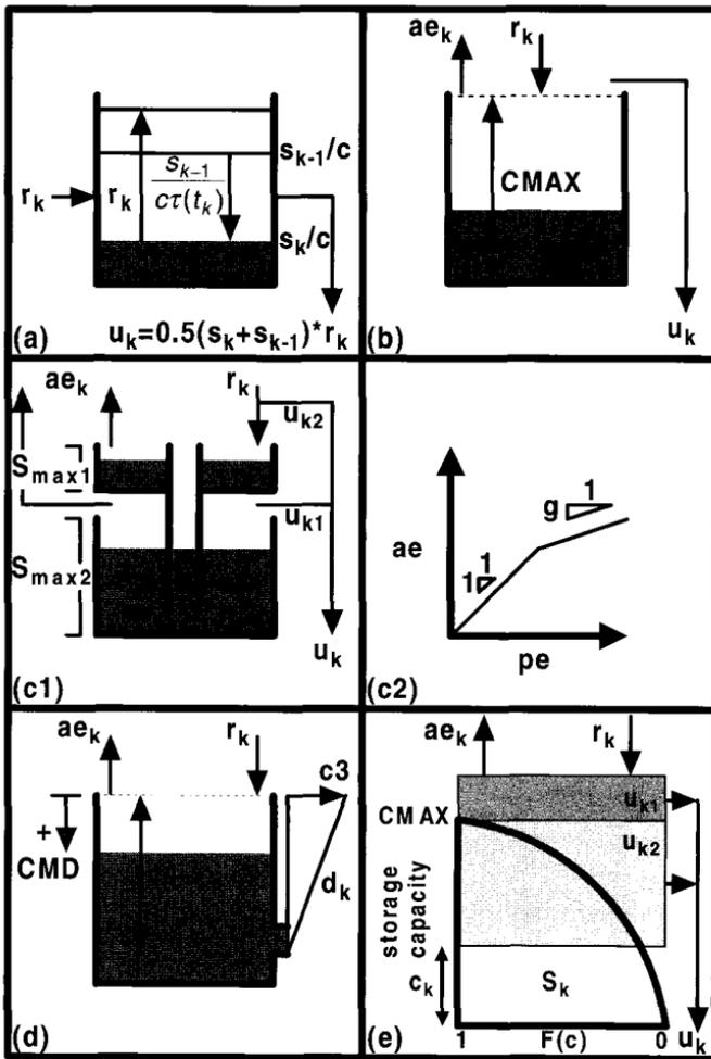
**Fig. 4.25** Table showing the soil moisture accounting ‘component library’ used in the application example. The components are: (a) catchment wetness index (cwi), (b) simple bucket (buc), (c1) and (c2) Penman structure (ic1), (d) catchment moisture deficit (cmd), and probability distribution of soil moisture stores (pdX). (From Wagener *et al.*, 2002; reproduced with permission of the American Geophysical Union)
