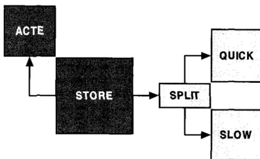
**Fig. 5.2** Schematic description of a general model structure with components (parameters) describing the actual evapotranspiration (ACTE), the storage volume, (STORE), the split between quick and slow response (SPLIT), and the quick and slow response residence times.
