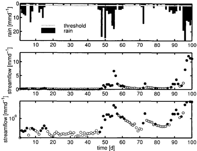
**Fig. 3.14** A hundred day period of Medway streamflow and rainfall segmented using a scheme modified from Boyle *et al.* (2000). The dots indicate time steps classified as driven (black), non-driven quick (grey), and non-driven slow (white). (Reproduced from Wagener *et al.*, 2002a; with permission of Water Resources Publications LLC.)
