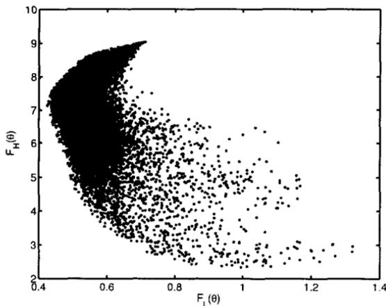
**Fig. 2.3** Model population resulting from a Monte Carlo simulation plotted in the 2-dimensional OF space.  $F_L$  is the RMSE for the part of the hydrograph classified as low flow;  $F_H$  is the RMSE for the high flow part. The optimum value for both functions is in the bottom left corner.
