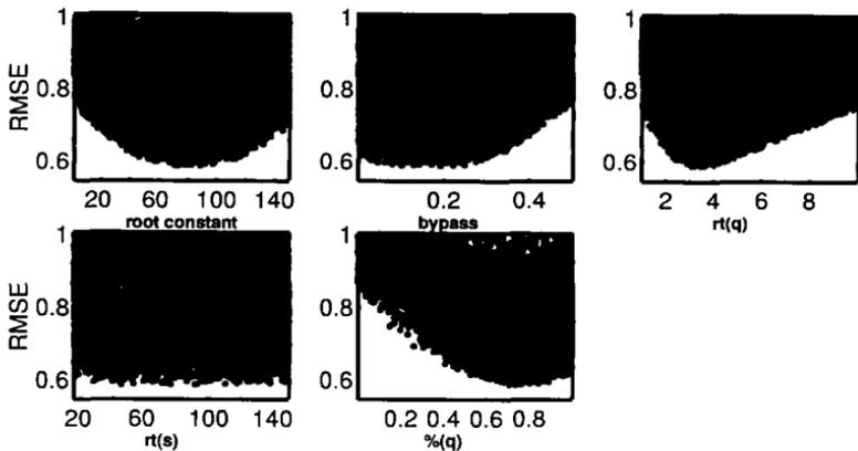
**Fig. 4.19** Dotty plot showing results of the uniform random search using 20000 samples utilizing the whole six-year period available. Lower values of the Root Mean Squared Error (RMSE) objective function indicate better performing parameter values. Only parameter sets producing an RMSE below  $1\text{mm d}^{-1}$  are shown. (From Wagener *et al.*, 2003a; reproduced with permission of John Wiley & Sons, Inc.)
