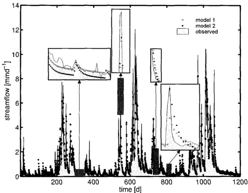
**Fig. 3.9** Plot showing predictions using two different parameter sets with an identical model structure. Both realizations yield similar values of the NSE measure (0.82), but show differences in fit when the response is analysed closely. (Reproduced from Wagner *et al.*, 2002a; with permission of Water Resources Publications LLC.)
