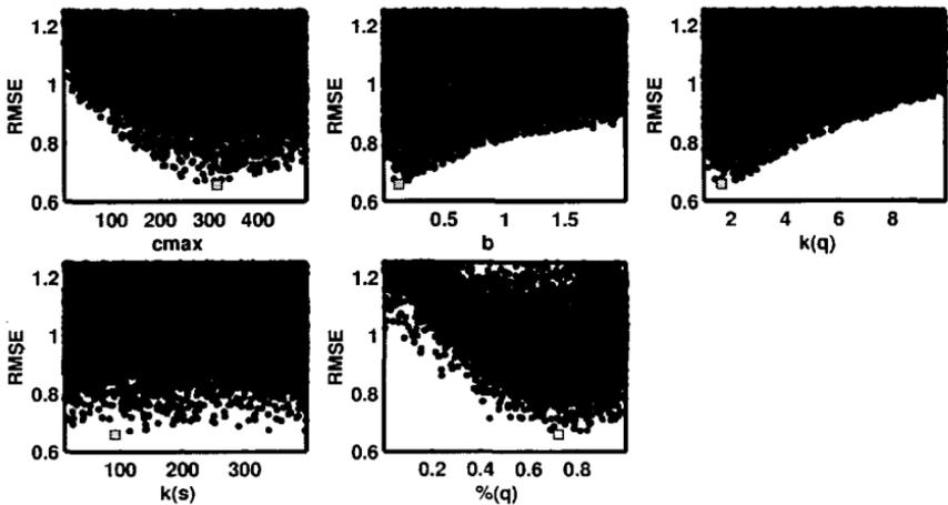
Fig. 5.14 Dotty plot for the test catchment, the Teise@Stonebridge. Result based on uniform random sampling with 10,000 parameter sets. The best parameter values are indicated by rectangles.
