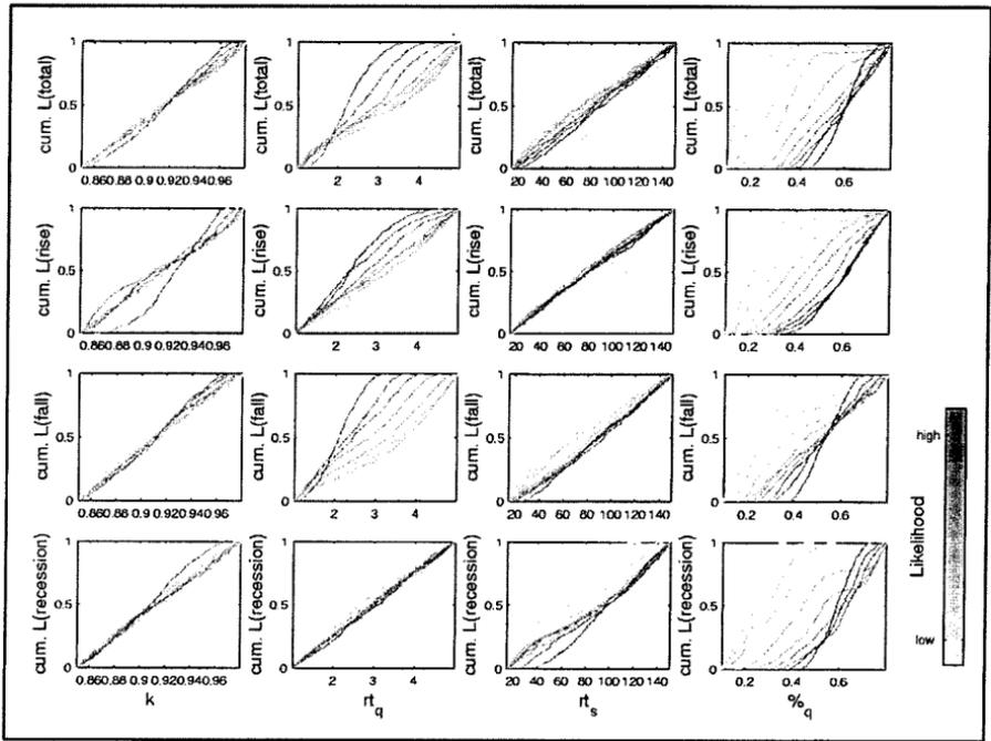
Fig. A.12 Visualization of changing sensitivity using extended RSA plots. The parameters are the API decay parameter  $k$ , the two residence times ( $rt_q$  and  $rt_s$ ) and the percentage quick flow ( $\%q$ ).
