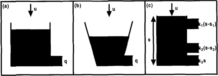
**Fig. 3.7** Conceptual routing components available in the RRMT: (a) linear; (b) non-linear (example); and (c) leaky catchment structure.
