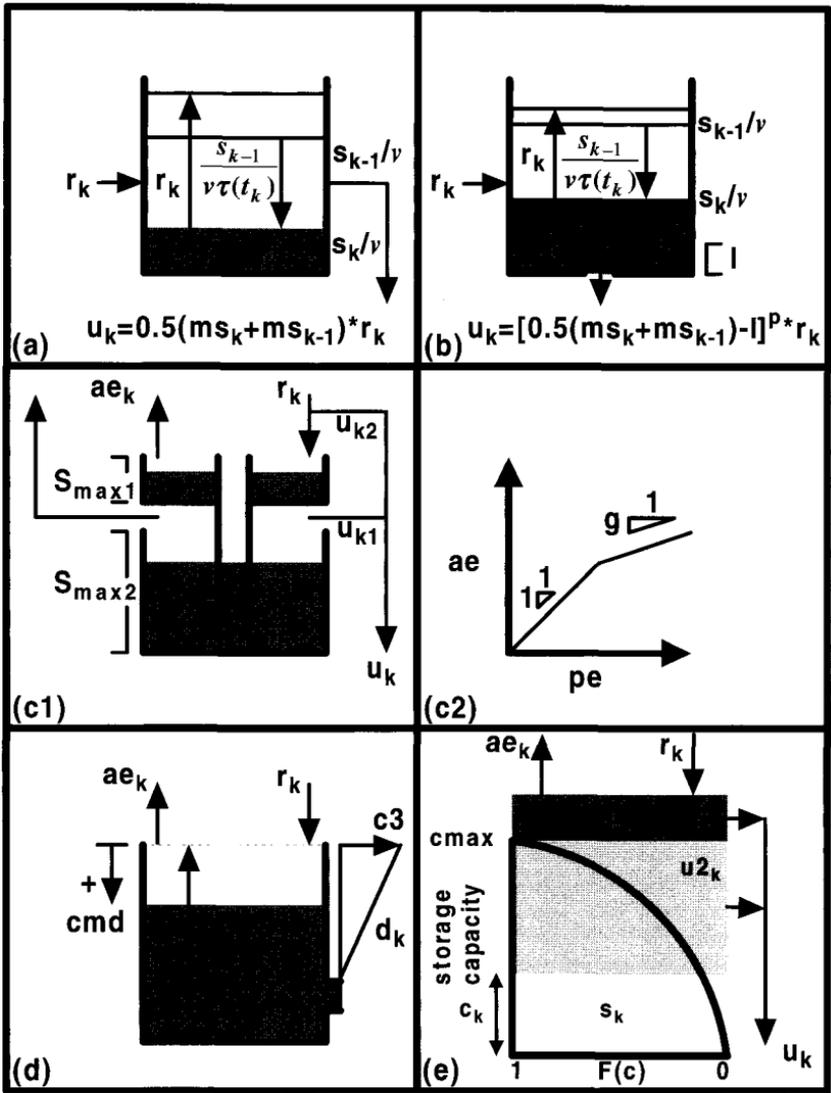
**Fig. 3.3** Schematic plots of the different moisture accounting modules available: (a) catchment wetness index (cwi), (b) modified cwi, (c1) conceptual Penman model structure, (c2) Penman drying curve, (d) catchment moisture deficit model structure (cmd), (e) storage capacity distribution function.
