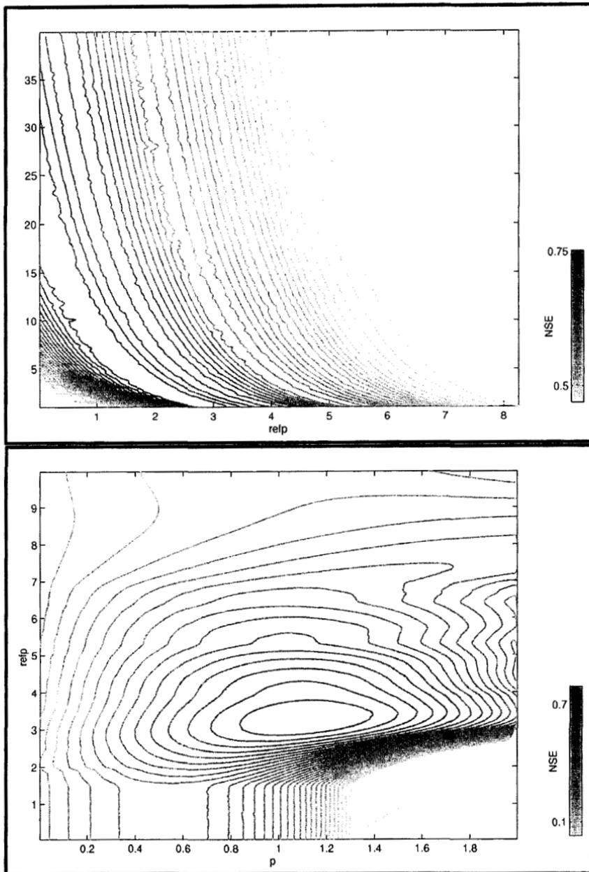
Fig. A.5 Two-dimensional MCAT plots show the interaction between two parameters. The top plot shows a poorly identified parameter that was subsequently removed.
