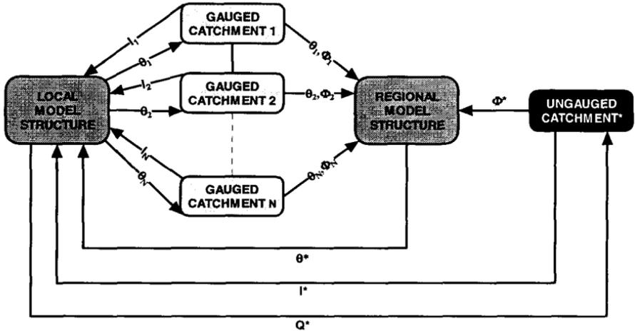
Fig. 5.1 The idea of conceptual parameter regionalization. Where  $\Phi$  are catchment characteristics,  $Q$  is the streamflow,  $\theta$  are model parameters and  $I$  are input time-series.
