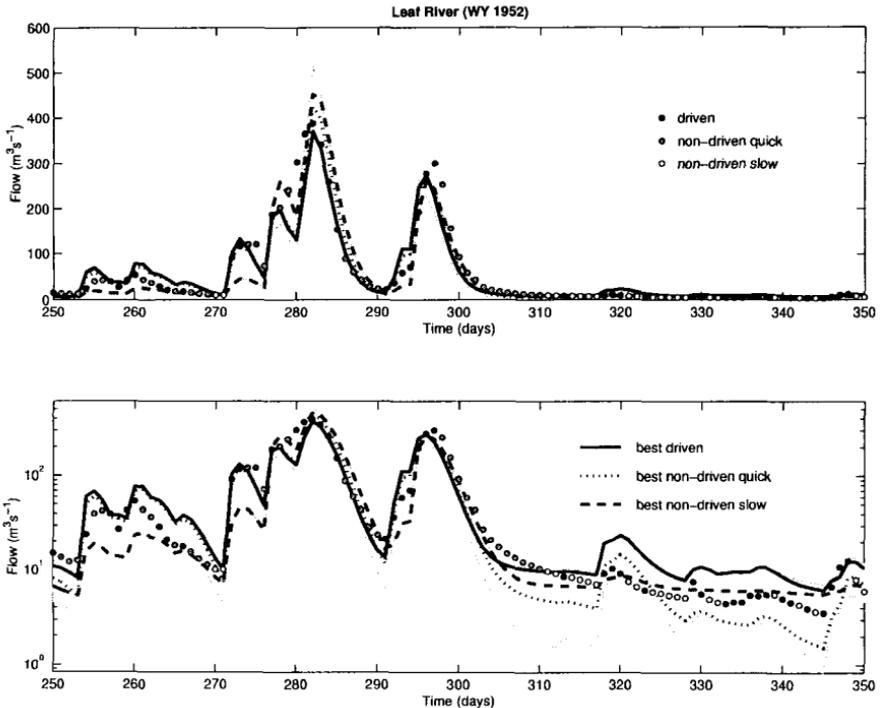
**Fig. 4.15** Hydrograph range produced by the 500 Pareto solutions (grey region), and the output from the best parameter sets for the different measures on normal (1<sup>st</sup> row) and on logarithmic scale (2<sup>nd</sup> row). The observed time-series is shown as circles. (Figure by Douglas P. Boyle, from Wagener *et al.*, 2001; reproduced with permission of the European Geosciences Union)
