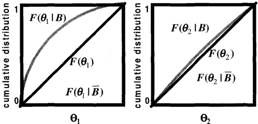
**Fig. 3.11** Cumulative distributions of initial ( $F(\theta_x)$ ), 'behavioural' ( $F(\theta_x | B)$ ) and 'non-behavioural' ( $F(\theta_x | \bar{B})$ ) populations for a sensitive parameter  $\theta_1$ , and a (conditionally) insensitive parameter  $\theta_2$ .
