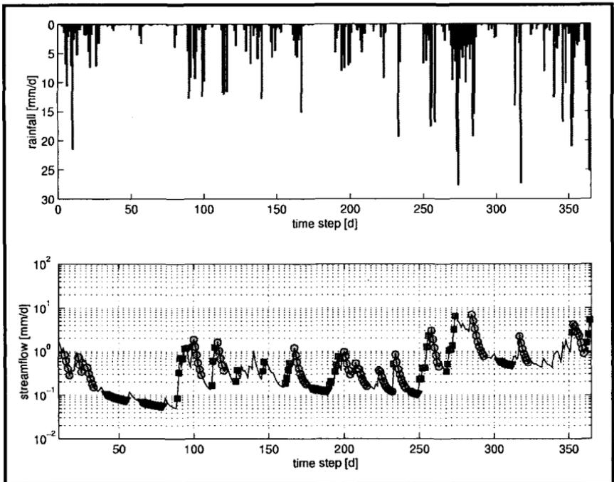
Fig. A.11 Measured rainfall and segmented synthetic flow used.
