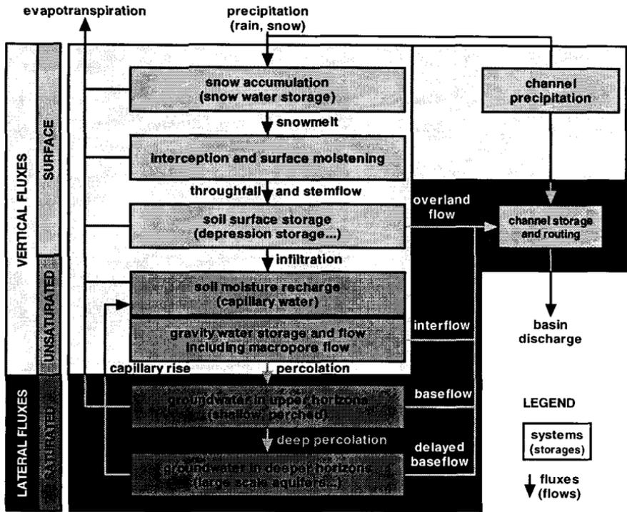
Fig. 2.1 Schematic presentation of hydrologic processes in a catchment modified from Becker (1992).
