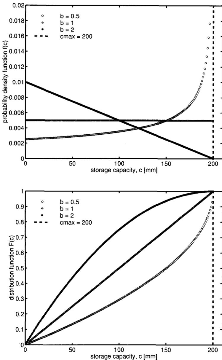
**Fig. 3.5** Pareto distribution of storage capacity. The probability density function is shown at the top, the distribution function at the bottom.
