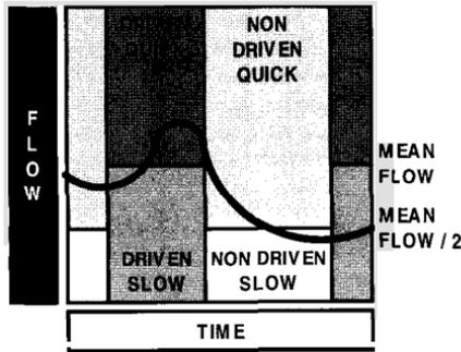
Fig. 4.26 Segmentation scheme used to derive multiple objective functions describing the model performance during different response modes.
