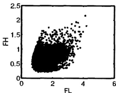
**Fig. 5.7** Scatter plot showing a model population based on 10000 samples from uniform parameter distributions projected into a 2-dimensional OF space. The two OFs are the RMSE utilizing the residuals at time steps during which the observed flow is respectively above (FH) or below (FL) the mean flow.
