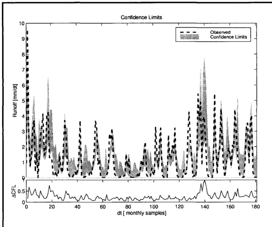
**Fig. A.4** Plot showing 95% confidence limits, calculated in the Box-Cox transformed space. The graph is an example taken from the regionalization study.
