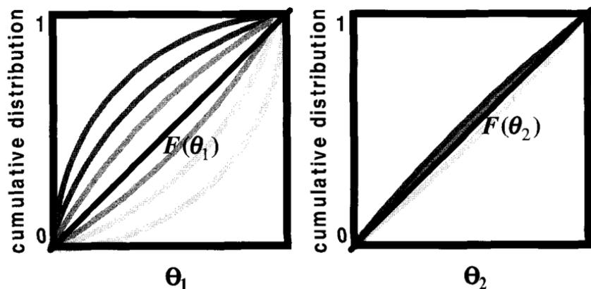
Fig. 3.12 Schematic Regional Sensitivity Analysis plot using the modified version of Freer *et al.* (1996). A sensitive parameter is shown in the left plot, while the right one shows an insensitive one.
