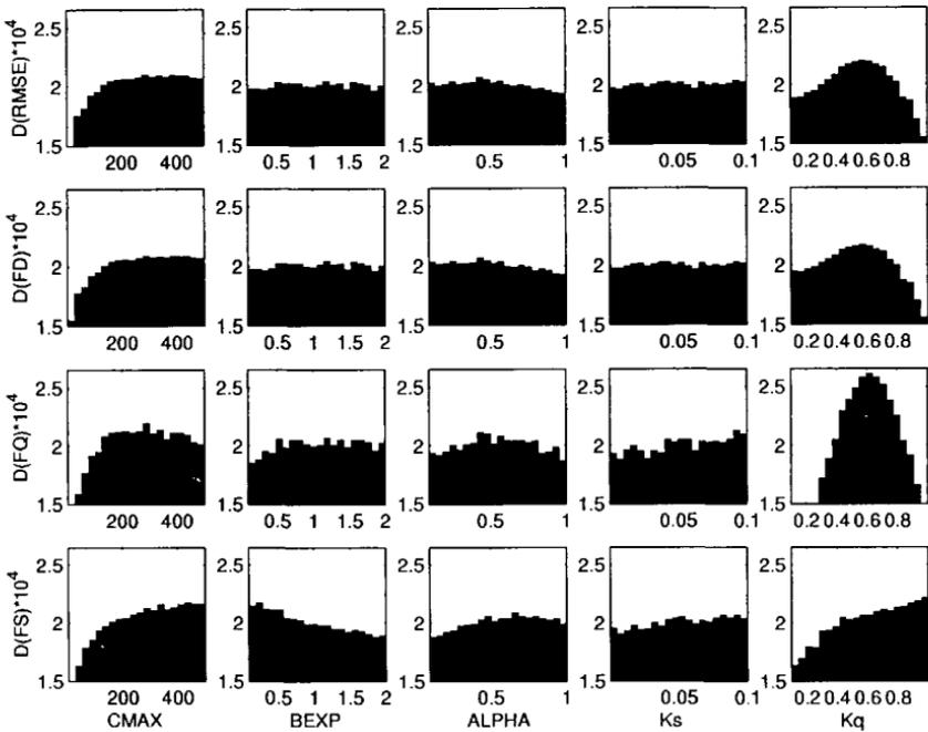
**Fig. 4.13** The objective functions are rescaled so that the best performing parameter assumes the highest value and the sum of all values equals one. Splitting each parameter range subsequently into 20 bins of equal width and calculating the sum of all measures in each container leads to the parameter density (D) distributions shown. (From Wagener *et al.*, 2001; reproduced with permission of the European Geosciences Union)
