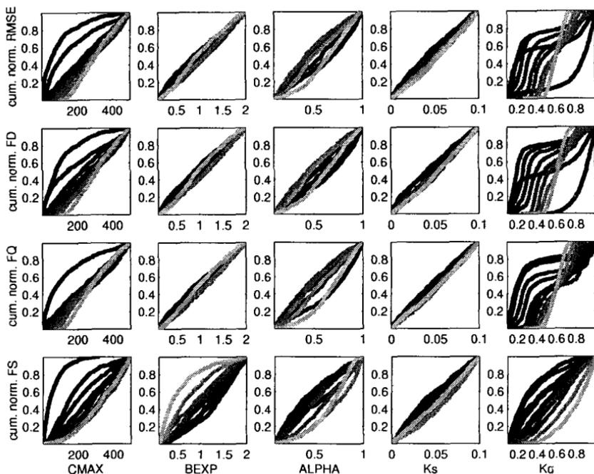
**Figure 4.12** Regional Sensitivity Analysis plots showing the varying sensitivity of the model parameters when using different objective functions. (From Wagener *et al.*, 2001; reproduced with permission of the European Geosciences Union)
