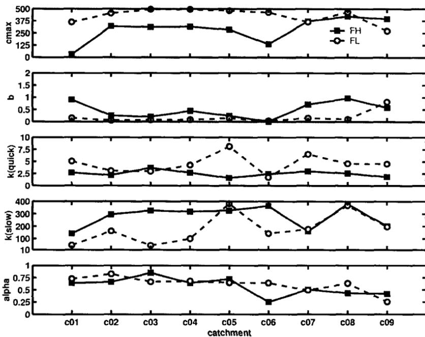
**Fig. 5.8** Variation in optimum parameter values for two different OFs representing two different modelling purposes. The two OFs are the RMSE utilizing the residuals at time steps during which the observed flow is above (FH) or below (FL) the mean flow respectively. The model structure applied is pd4-2pll.
