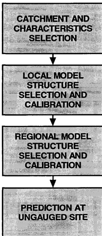
Fig. 2.4 Conventional procedure for regional rainfall-runoff modelling.
