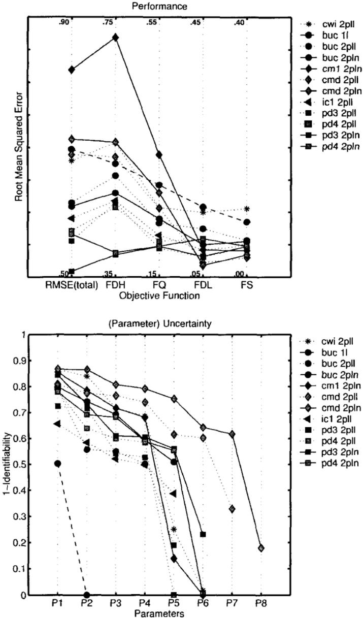
Fig. 4.27 Results of the model structure comparison. (From Wagener *et al.*, 2003b; reproduced with permission of the American Geophysical Union)
