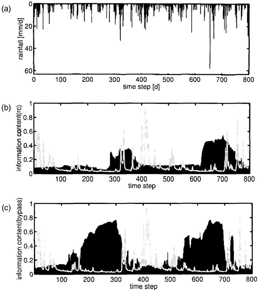
**Fig. 4.20** The information content of the data over a two-year period (days 950 to 1750). Graph (a) shows the precipitation input over the considered period. The remaining plots show the result for the different parameters (black bars). The grey line is the streamflow, normalized with respect to its maximum value. (From Wagener *et al.*, 2003a; reproduced with permission of John Wiley & Sons, Inc.)
