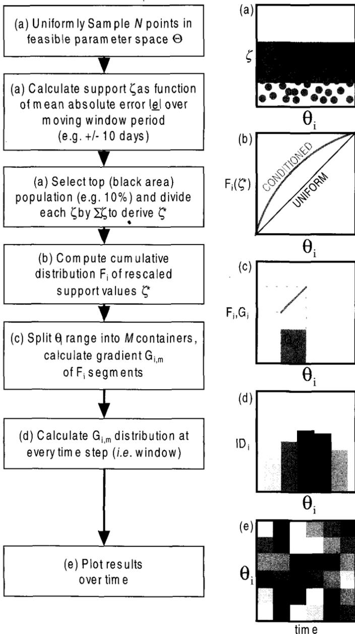
**Fig. 4.6** Schematic description of the DYNAMIC Identifiability Analysis (DYNIA) procedure.
