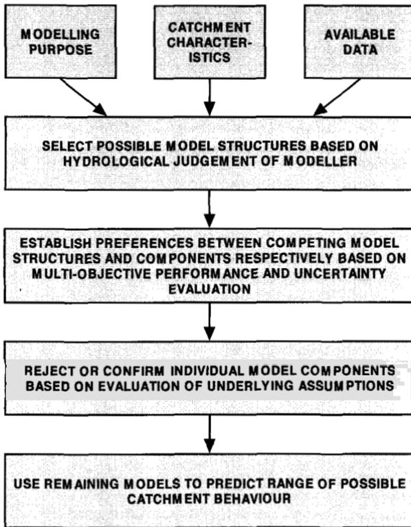
**Fig. 4.8** The proposed modelling framework. (From Wagener *et al.*, 2003b; reproduced with permission of the American Geophysical Union)
