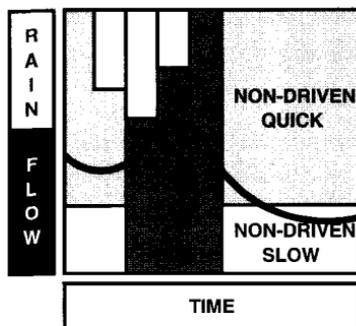
**Fig. 4.11** Hydrograph segmentation into three components based on different response modes of the catchment system, i.e., ‘driven’ (QD - dark grey), ‘non-driven quick’ (QQ - light grey) and ‘non-driven slow’ (Q<sub>S</sub> - white) flow. (From Wagener *et al.*, 2001; reproduced with permission of the European Geophysical Union)
