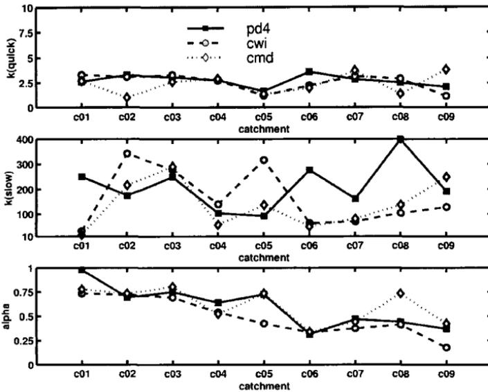
**Fig. 5.6** Comparison of  $k(\text{quick})$  [d],  $k(\text{slow})$  [d] and  $\alpha$  [-] values for the pd4-2pll, cwi-2pll and cmd-2pll model structures. Values shown are optimal with respect to the RMSE criterion.
