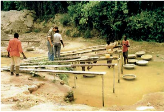
Fig. 150 Chutes for liquid clayey gold mud used in artisanal mining in the Ashanti region
