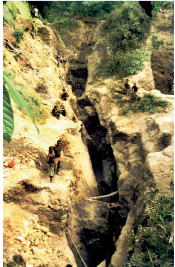
Fig. 149 A pit for artisanal gold mining in the Ashanti Region
