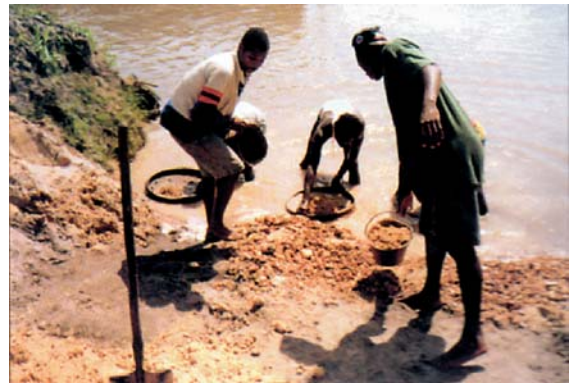
Fig. 158 Screening of diamond-bearing gravel by artisanal miners in the Kerouane region
