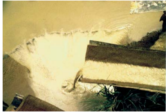
Fig. 152 The siphon of a liquid gold mud delivering chute in the Ashanti region
