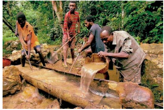
Fig. 88 Artisanal processing of coltan ore in eastern DRC
