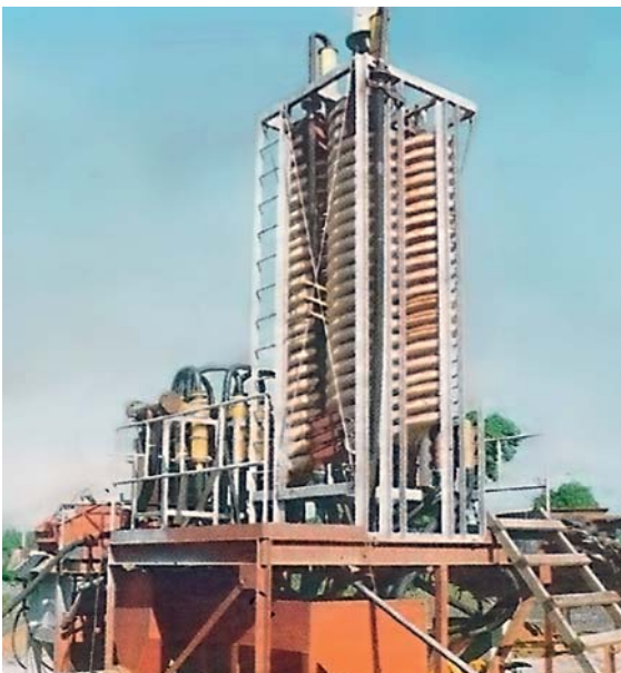
Fig. 177 Machinery to be used for the production of ilmenite, rutile and zircon from beach sands at Kwale
