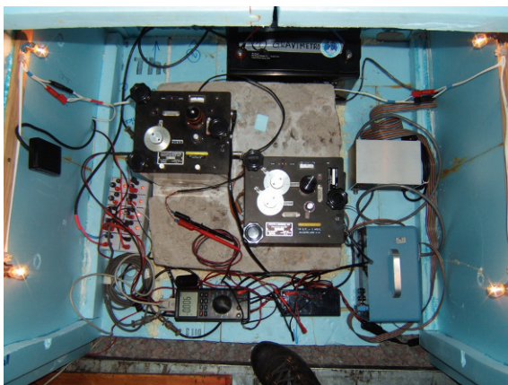
Fig. 11 Set-up of the instruments at a grounded pillar within the gravimeter hut, Belgrano II: L&R G-748 (left), L&R D-193 (right)
