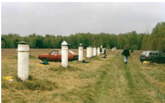
Fig. 2 Examination of vertical component differences in phase centres of 6 different antennae
