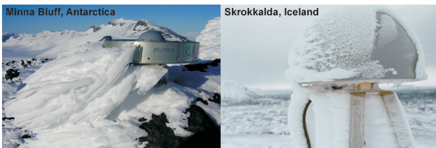
Fig. 10 (left) Rime ice build up on unprotected GPS antenna at Minna Bluff, Antarctica. The site is prone to low clouds and high wind speeds. Photo by Bradish Johnson, USGS. (right) Rime ice build up on a GPS antenna equipped with a short SCIGN dome radome at Skrokkalda, Iceland, photo by Halldór Geirsson, modified from SCIGN website. Rime can be a difficult problem
