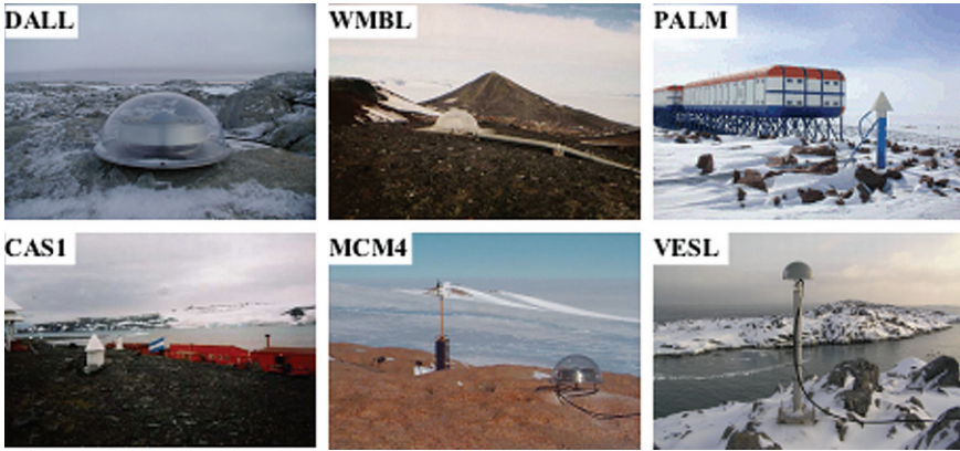
Fig. 7 Different types of antenna mounted on Antarctic GNSS stations
