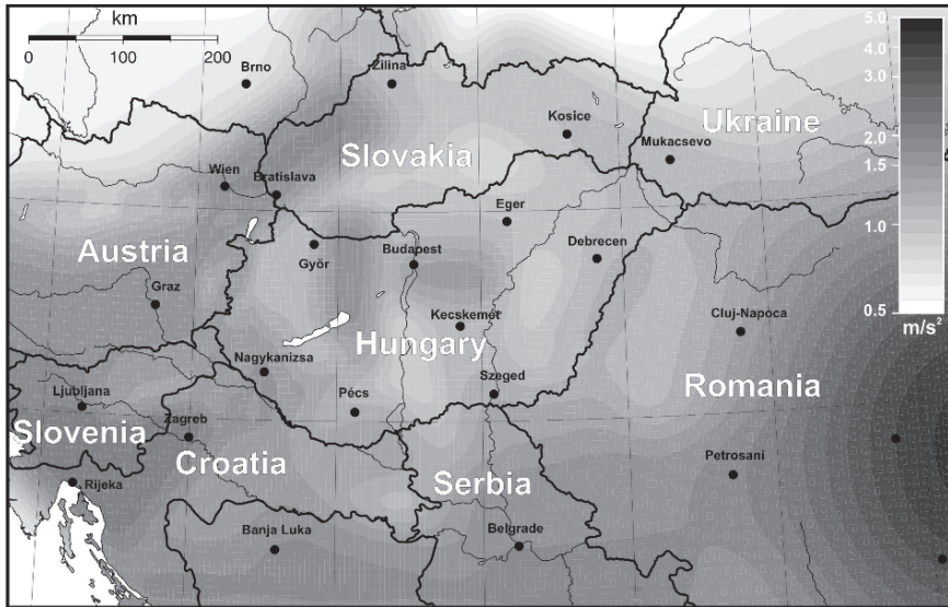
Figure 7 Seismic hazard in the Pannonian basin region. Expected peak ground acceleration in \text{m/s}^2 (10% probability of exceedance in 50 years, 475-year return period)
