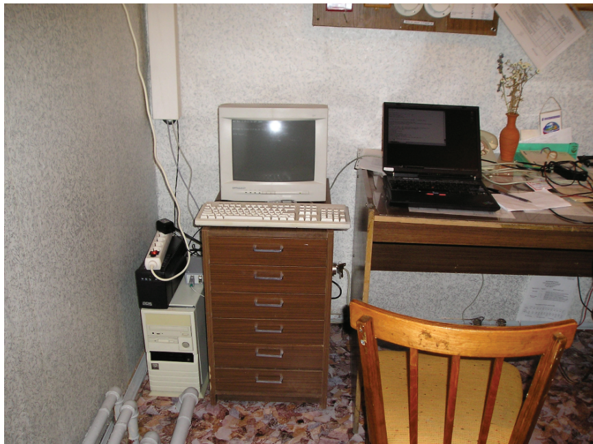
Figure 5 Data logger and the center for the station operation. A laptop is used for the real time data display while the data logger has no graphic interface. Photo taken at the BELME station in Karelia, NW Russia
