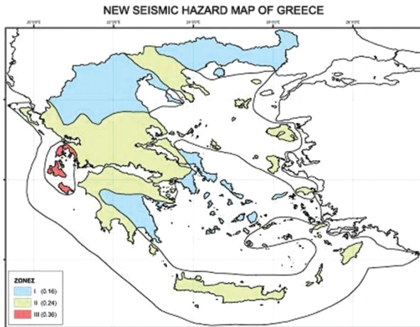
Figure 9 The new official seismic hazard map of Greece since 1-1-2004. Only three zones of 0.16g, 0.24g and 0.36g are included in the new version
