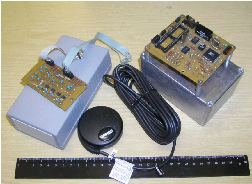
Figure 4 Station parts: Time Synchronization Device (left), GPS-clock and ADC (to the right)
