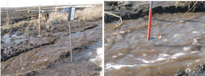
**Fig. 6** Determining the speed of a water stream using a “GR-99” hydrological rotator
