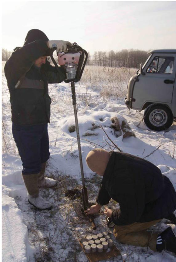
recognized visually, but also estimated from data on soil temperature and moisture content (Tanasienko and Chumbaev 2010). Therefore, it is necessary to set up a thermometric plot near each runoff plot. We obtained reliable data using small (roughly coin-sized) electronic temperature recorders (Thermochron iButton Device 2013).
