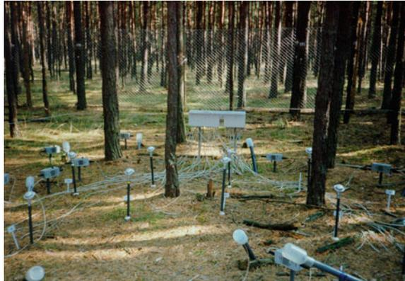
data logger or notebook computer. In our investigations, readings are taken at hourly intervals. The systems are powered by batteries. The hydrological measuring fields are positioned to cover representative areas under the tree crowns and also areas close to the trunks (Müller 2002, 2006).
