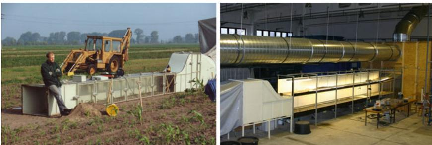
Fig. 10 Mobile and stationary wind tunnel used by the author
