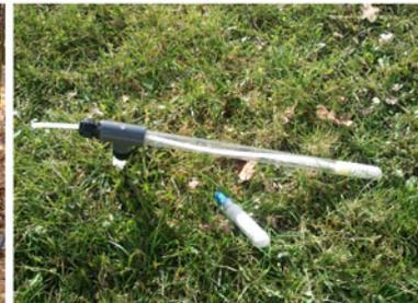
**Fig. 7** **a** Measuring field with suction probes to collect soil solution at different soil depths in a pine-beech mixed stand. **b** A suction probe with ceramic cup
