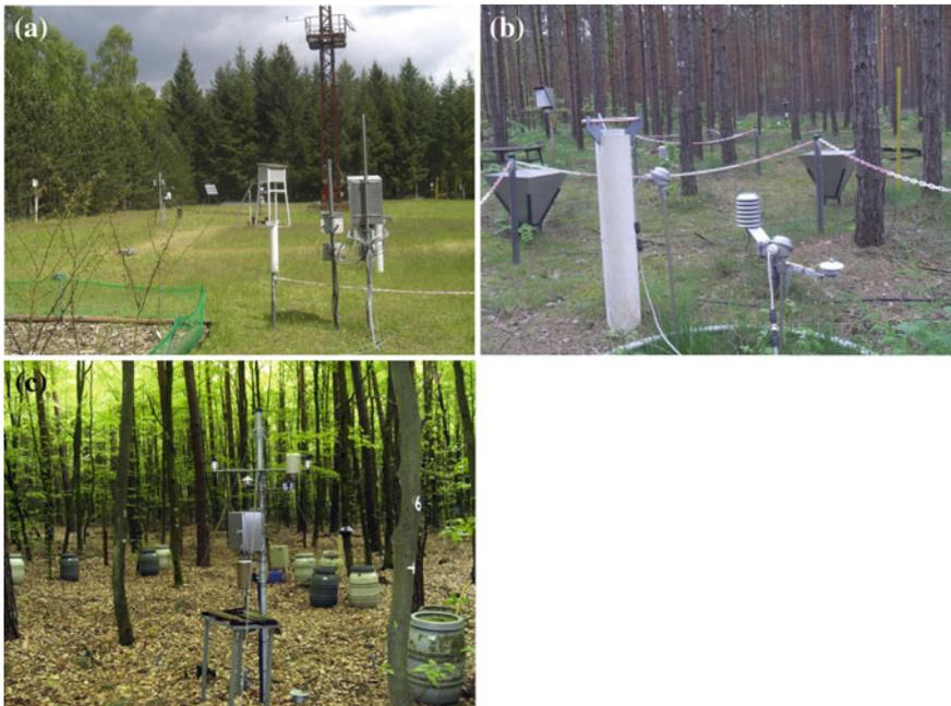
**Fig. 3** Well-engineered forest monitoring plots operating in the German Forest Monitoring Network, Eberswalde site. The open field plot **a** consists mainly of meteorological instruments, while the plots in needle-leaf stands **b** and broadleaf stands **c** consist of tensiometers, TDR and FDR moisture probes, suction probes, lysimeters, dendrometers and more
