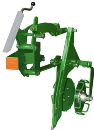
drill (DMC system) was also tested in Pervomaisky, which is also equipped with individual depth control on the chisel openers (Fig. 22).
