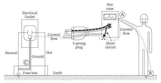
**FIGURE 18.3:** Grounded power and grounded equipment. Most of the fault current travels to the ground (point A to point C—lesser resistance) with only a small portion going through the individual (point A to point B— higher resistance).
