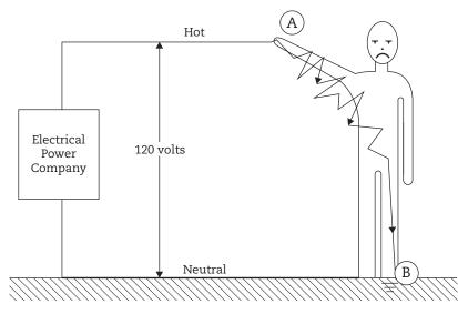
**FIGURE 18.2:** Completion of an electrical circuit through the body by touching a single hot wire (point A) while in contact with the ground (point B).
