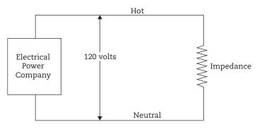
**FIGURE 18.1:** An alternating current (AC) circuit with 120 volts of potential difference between the hot and neutral side of circuit.
