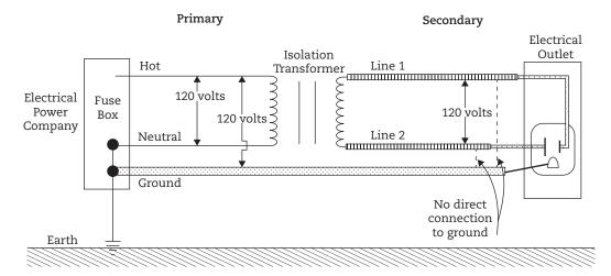
FIGURE 18.4: Diagram showing how the isolation monitor provides ungrounded electrical power to the secondary side.
