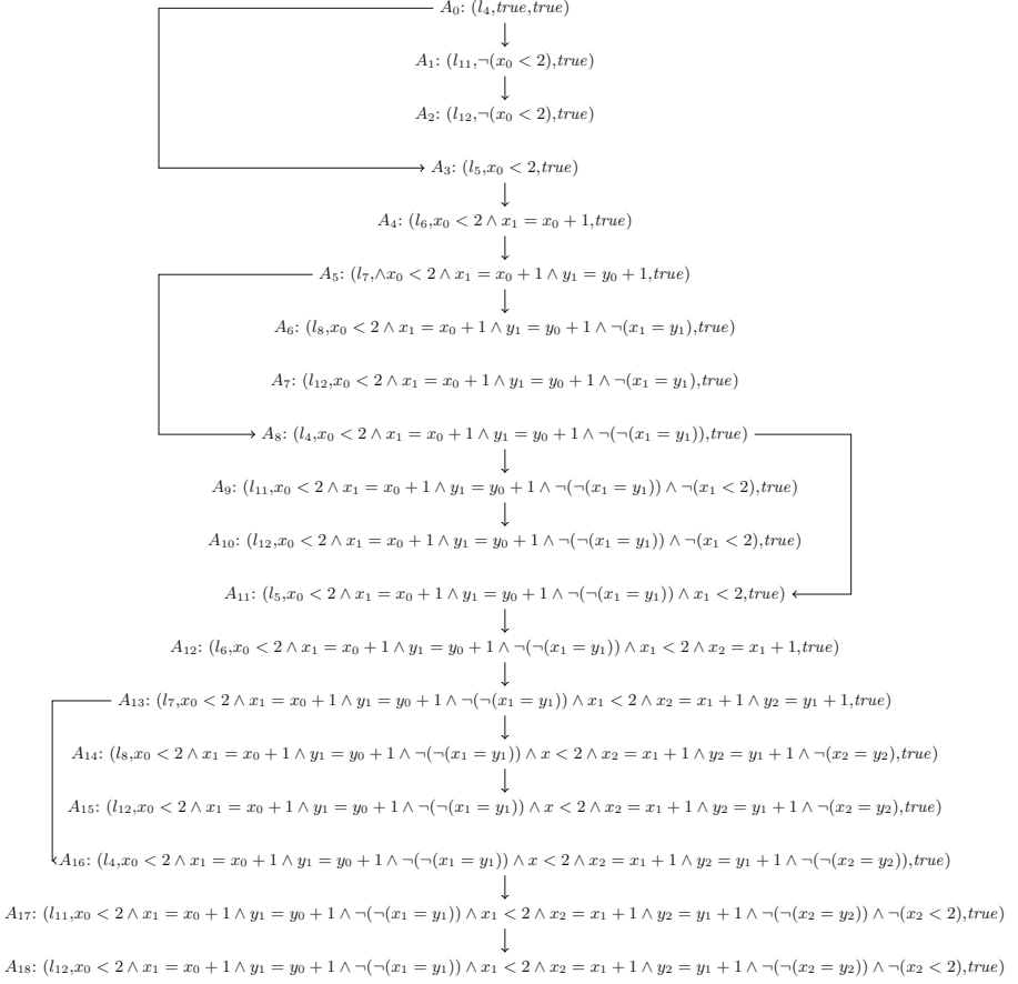
Fig. 4. ARG fragment for the inductive-step case of k -induction applied to the example of Fig. 2
