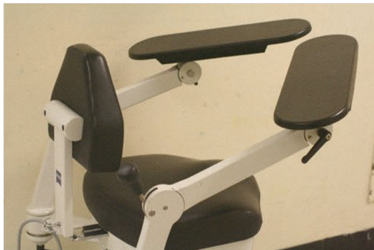
Fig. 93.7 Carl Zeiss Meditec (Dublin, CA) microsurgeon chair with individual full arm supports and powered vertical height refinement, allowing total arm support and neutral ergonomic surgeon positioning during prolonged microsurgical cases.
