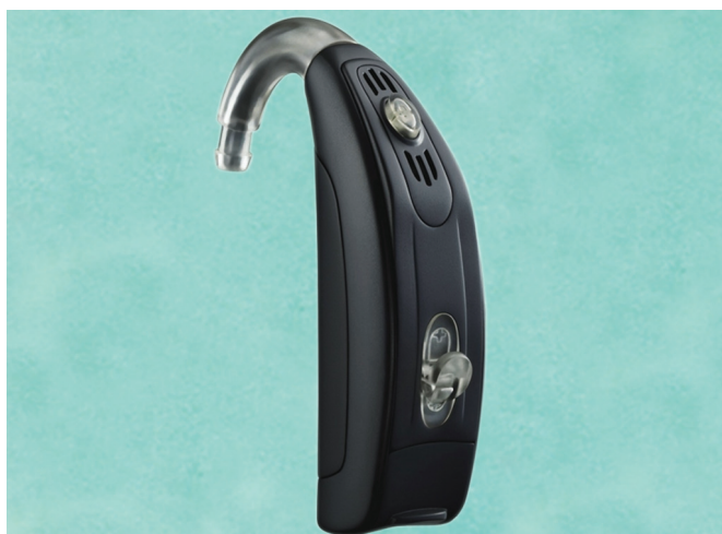
Fig. 31.3: Behind-the-ear (BTE) hearing aid. Photo courtesy of Unitron Hearing.
