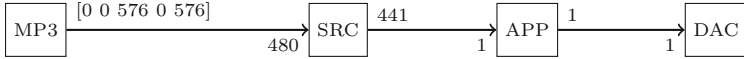
Fig. 1. A CSDF graph for the MP3 playback application [10]. Production and consumption rates are shown on the edges.
