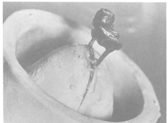
Fig. 18.5 Wax pattern on U-shaped sprue-former, held in crucible-former with split top. The addition of reservoirs 1.0 mm from the pattern will prevent suck-back of gold when solidifying.
