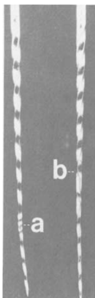
Fig. 25.25 The effects of over-strain on reamers. (a) The reamer has jammed apically and, by continued torsion, has been twisted to a tight spiral. (b) After jamming, the reamer has been unwound by turning it in an anti-clockwise direction, unwinding the flutes. Both reamers are in imminent danger of fracturing.
