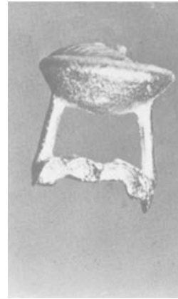
Fig. 18.4 Mal-location of sprues results in rounding of margins of the casting because the gold has to flow against gravity.
