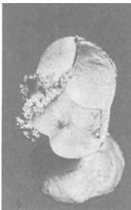
Fig. 18.27 Failure to cast owing to cracking of investment. Note the fins and bubbles which indicate disintegration of investment. Either the mix was too thin, or the investment was not set when the ring was put into the oven or the temperature was raised too quickly.
