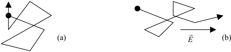
Figure 1.16. Trajectory of a carrier (a) in the absence and (b) in the presence of an electric field.
