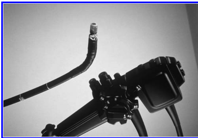
FIGURE 13.8 A picture showing the distal end of a radial scanning echoendoscope. This is a standard endoscope with oblique-forward viewing optics with an ultrasound transducer mounted on the distal tip. The ultrasound transducer is rotated 360° around the long axis of the scope producing a 360° image.
