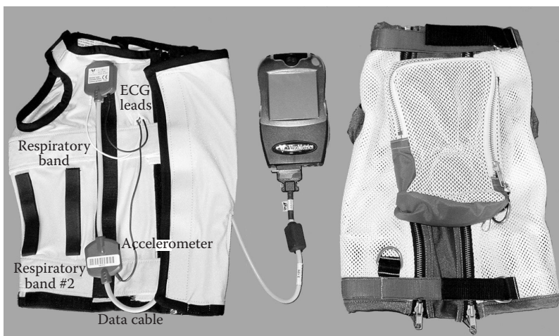
FIGURE 12.27 Complete LifeShirt System—the LifeShirt garment is on the left. The data recorder contains a removable flash memory card, the battery, and an interactive touch screen that can be used to mark study events (treatment, dosing, etc.), as well as to display waveforms for the evaluation of signal quality. The jacket on the back provides protection for the equipment and contains a pouch in which the data recorder is stored during recording periods. (Courtesy of A. Derchak, VivoMetrics, Inc.)
